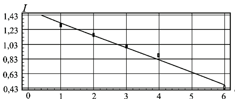
Figure. 1: Dependence of wear I from working time t without lubrication: points - experimental data, line - regression equation
