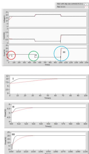
**Figure 6.** Comparison of FSS P&O (0.1V) and CSS P&O simulation results.
