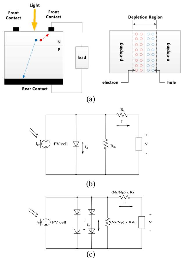
**Figure 1.** Scheme and equivalent circuits of photovoltaic cell. (a) PV cell operating principle, (b) PV cell equivalent circuit, and (c) PV module and array equivalent circuit.
