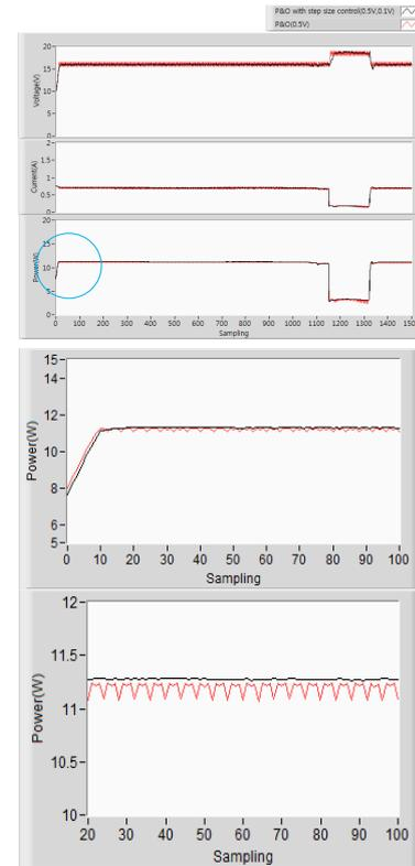
**Figure 7.** Comparison of FSS P&O (0.5V) and CSS P&O under partial shading experimental results.
