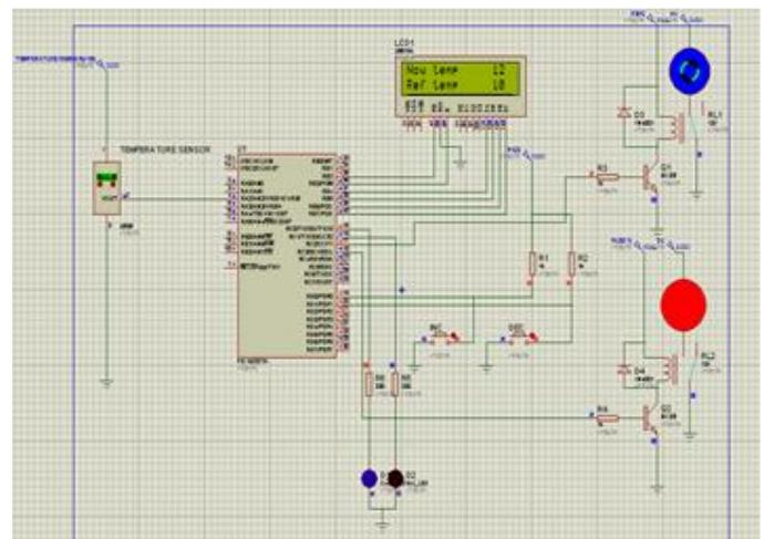
**Figure 6:** The completed circuit as shown in the simulation
