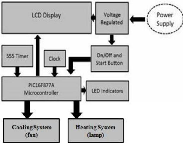
Figure 1: Block diagram for sensing system
