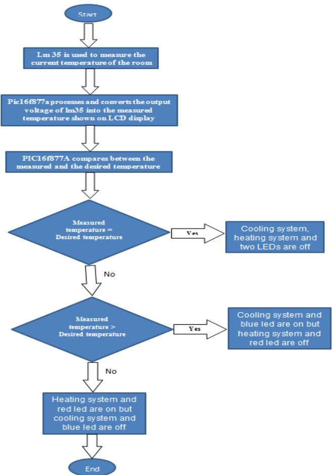
Figure 4: Flowchart of the system operation
