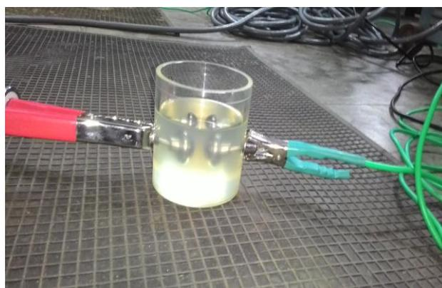
**Figure 3:** Arrangement to find out the Capacitance and Tan Delta of a sample
