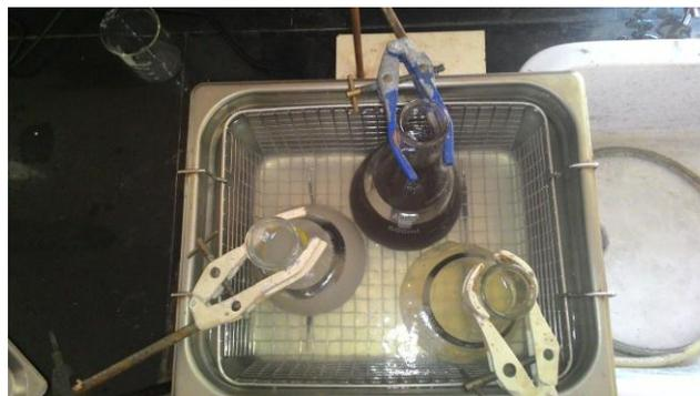
**Figure 1:** Arrangement of conical flasks inside the sonicator using holder
