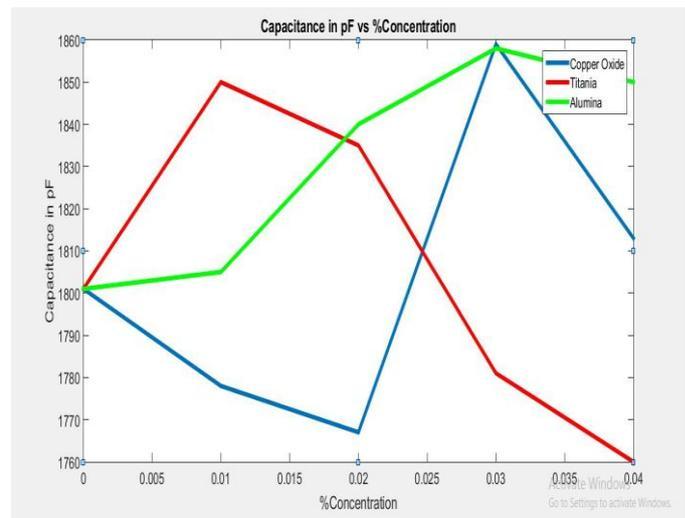
**Figure 5: Capacitance vs % Concentration**
