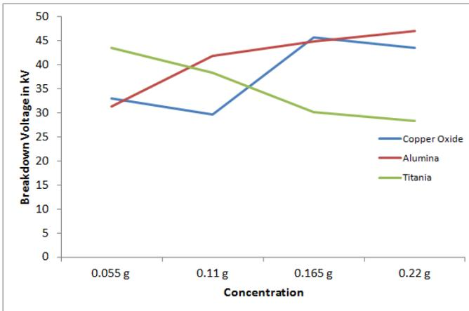
**Figure 6:** Breakdown Voltage vs Concentration
