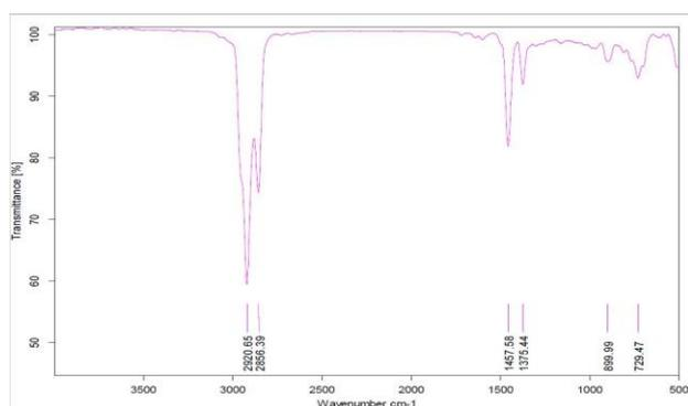
**Figure 3.2.2** FTIR spectra of oil - Polypropylene without catalyst
