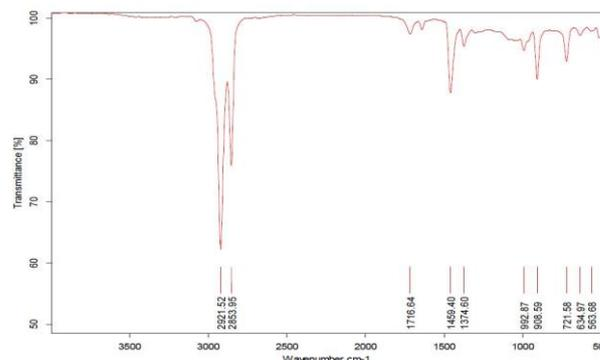
**Figure 3.2.4** FTIR of HDPE oil sample obtained after adding nickel oxide nano particles
