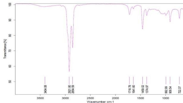
**Figure 3.2.3** FTIR of HDPE oil sample obtained after adding nickel nano particles
