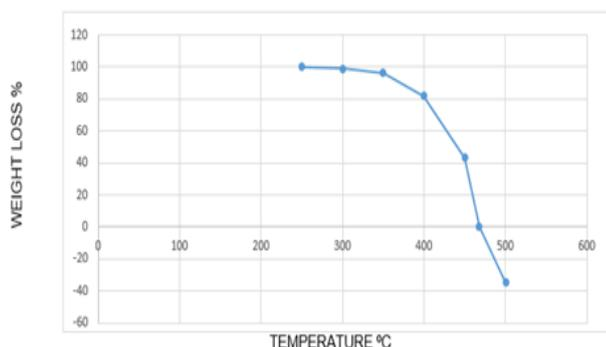
Figure 2.2.1 TGA Curve for Virgin HDPE
