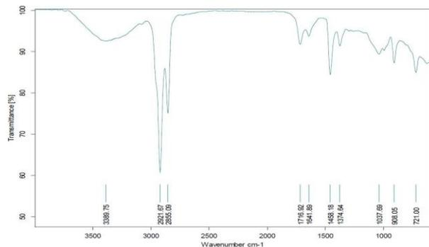
**Figure 3.2.1** FTIR spectra of oil - HDPE without catalyst
