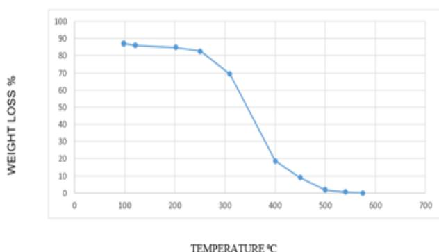
Figure 2.2.2 TGA Curve of Polypropylene
