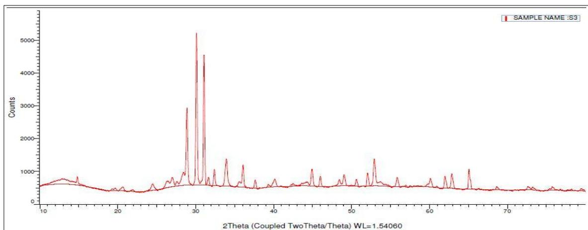
**Figure 3:** XRD results for Lead deposits
