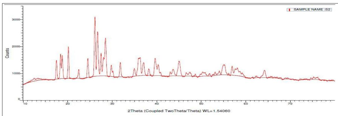
**Figure 2:** XRD results for Copper deposits
