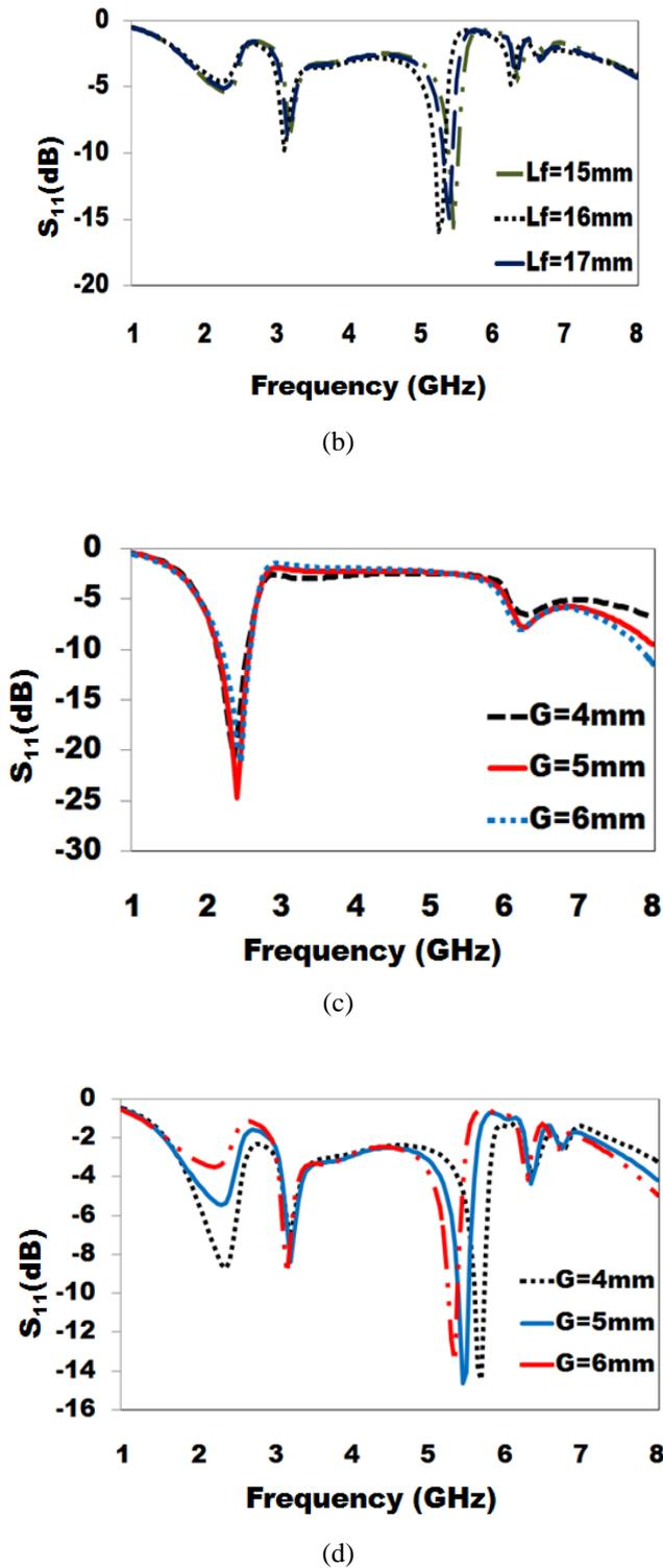
**Figure 2.** Parametric study of (a) Feed Length in OFF state, (b) Feed Length in ON state (c) Ground patch in OFF state and (d) Ground patch in ON state
