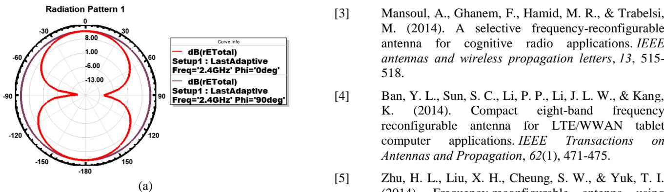
**Figure 6.** Simulated radiation pattern at (a) 2.4, (b) 5.45 GHz
