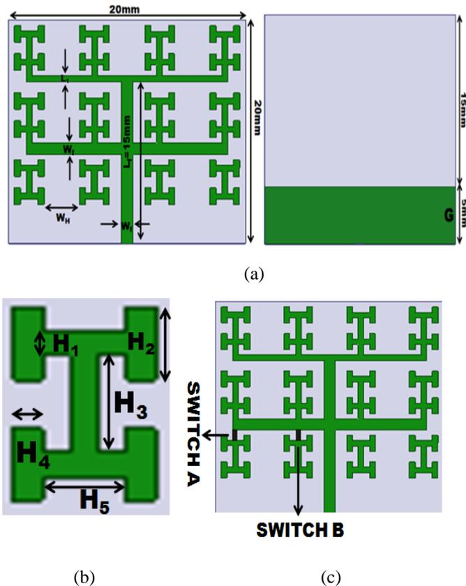
**Figure 1.** Structure of proposed reconfigurable antenna (a) Front patch & ground plane without switches, (b) H-shaped stub detailed geometry, (c) front patch with switches.
