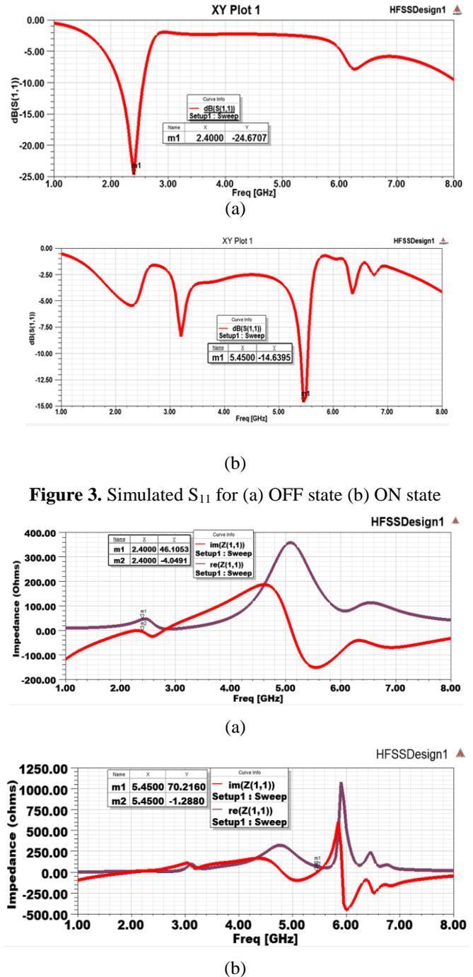
**Figure 4.** Simulated input impedance for (a) OFF state (b) ON state
