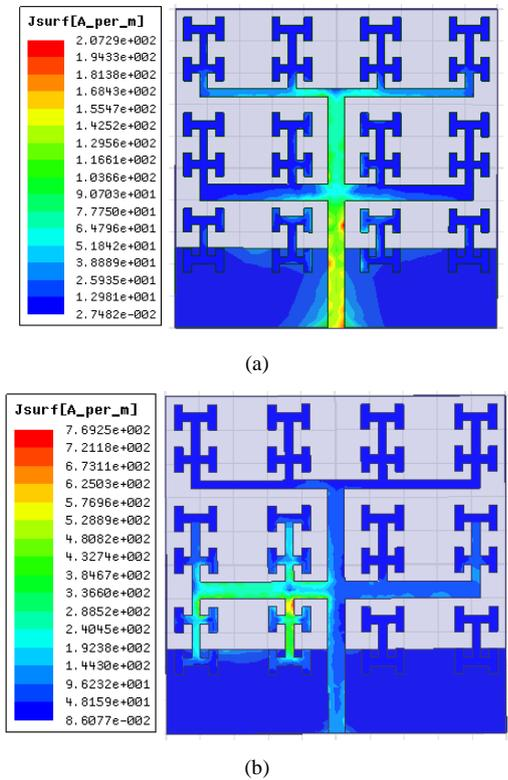
**Figure 5.** Current distribution at (a) 2.4, (b) 5.45 GHz
