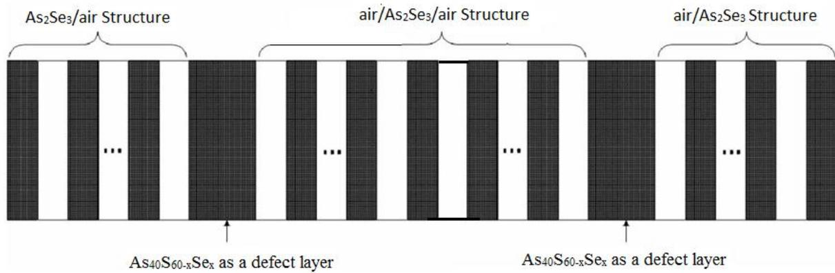
**Figure 2.** Schematic diagram of Two Defect layer in 1-D Photonic crystal
