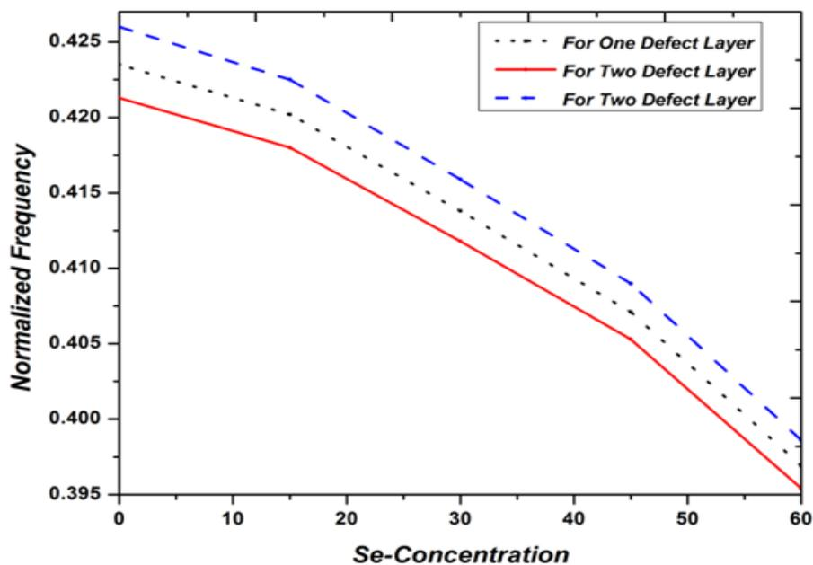
(b) Solid line for frequencies for left defect mode of two defect layer, dash line for frequencies for right defect mode of two defect layer and dotted line for frequencies for defect mode of one defect layer
