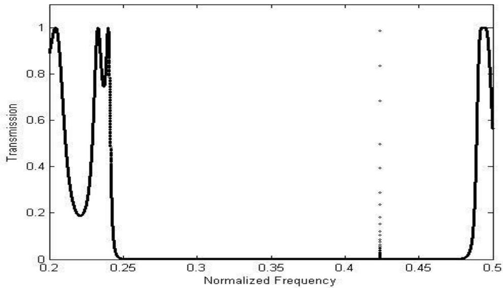
**Figure 4.** Transmission spectra for 1-D chalcogenide photonic crystal with one defect layer of  $As_{40}S_{60}$  of thickness  $d_c = 0.4a$ .
