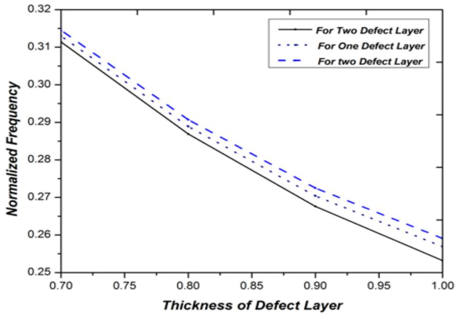
(a) Solid line for frequencies for left defect mode of two defect layer, dash line for frequencies for right defect mode of two defect layer and dotted line for frequencies for defect mode of one defect layer
