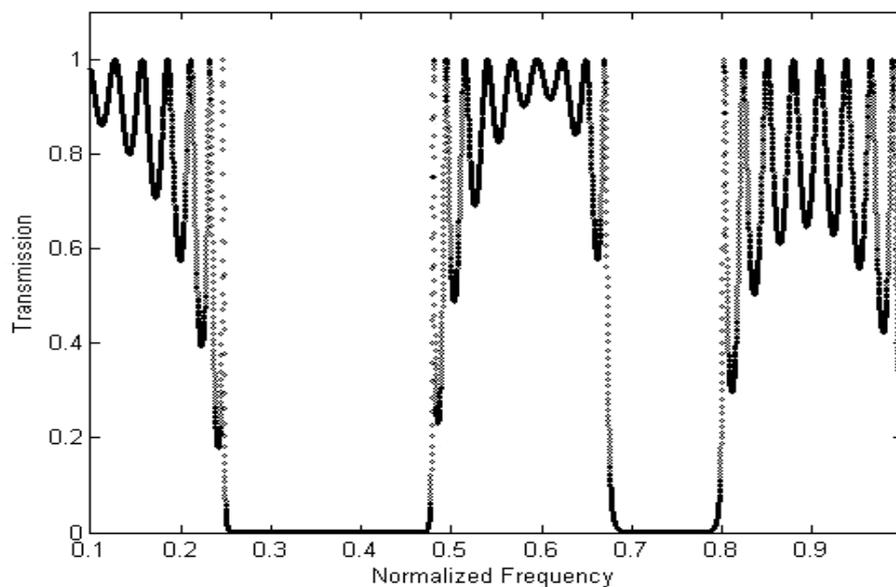
**Figure 3:** Transmission spectrum for  $As_2Se_3/air$  1-D multilayered structure without defect.
