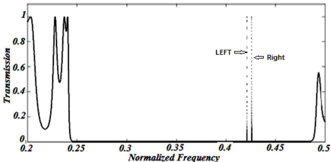
**Figure 5:** Transmission spectra for 1-D chalcogenide photonic crystal with two defect layer of  $As_{40}S_{60}$  of thickness  $d_c = 0.4a$ .
