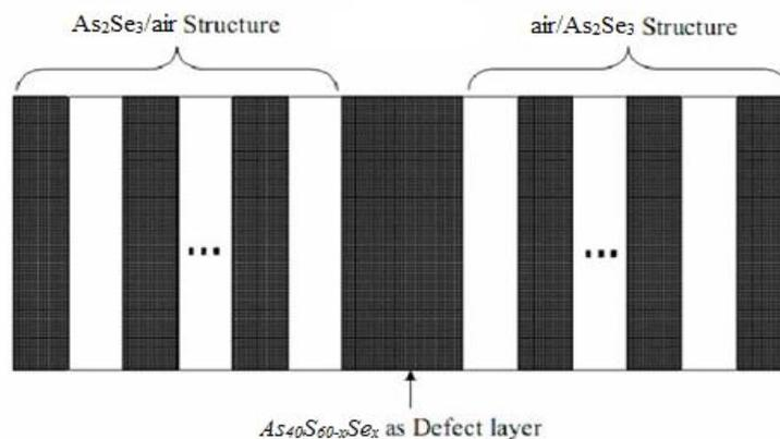
Figure 1. Schematic diagram of one Defect layer in 1-D Photonic crystal
