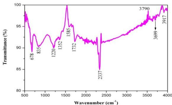
**Figure 3.** FTIR spectrum of NLBS0.0 glass (host glass)
