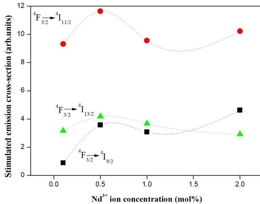
**Figure 6.** Variation of stimulated emission cross-section of Nd<sup>3+</sup> - doped LBS glasses for three different emission transitions
