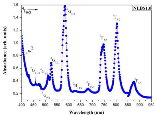
**Figure 4.** Absorption spectrum of NLBS1.0 glass along with the assignment of absorption bands
