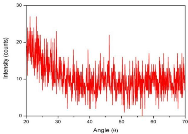
**Figure 2.** XRD pattern of NLBS0.0 glass (host glass)
