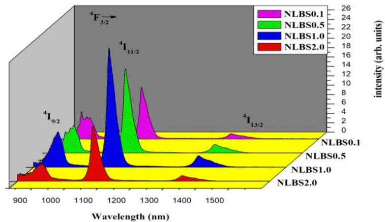
**Figure 5.** Photoluminescence spectra of NLBSX (X = 0.1, 0.5, 1.0 and 2.0 mol %) glasses
