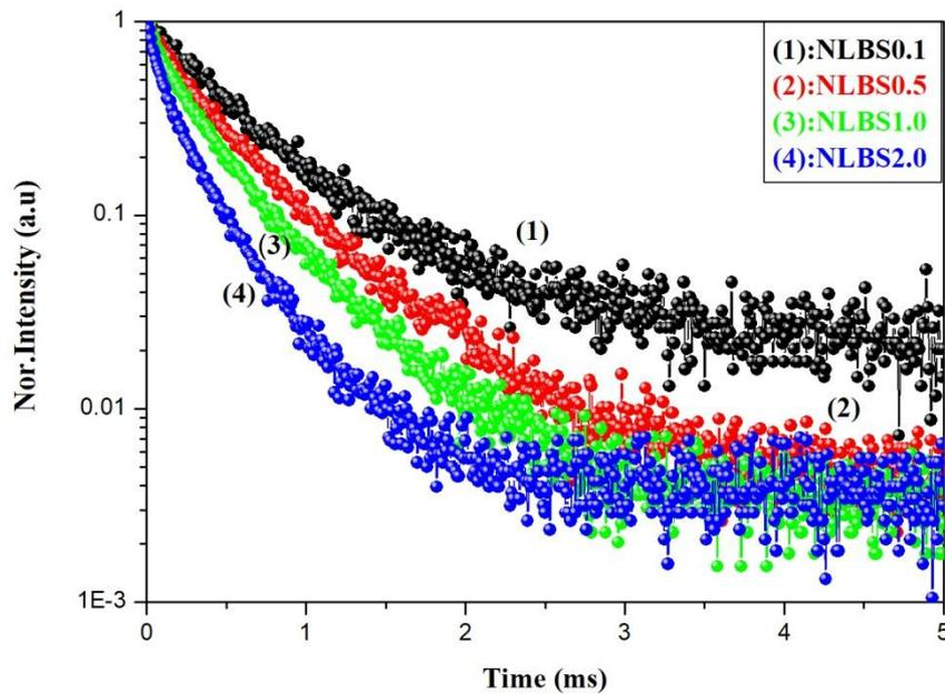
**Figure 7.** Photoluminescence decay profiles of  ${}^4F_{3/2}$  excited level for different concentrations of  $Nd^{3+}$  - doped LBS glasses
