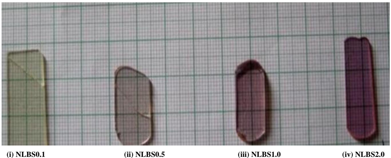
**Figure 1.**  $\text{Nd}^{3+}$  doped lead borosilicate glasses
