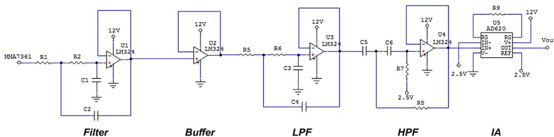
**Figure 3:** Signal conditioning circuit
