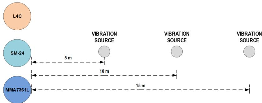
**Figure 5:** Acquisition design to obtain signal responses given by vibration sources in different distances
