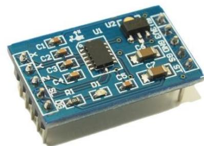
Figure 1: MEMS Accelerometer MMA7361L
