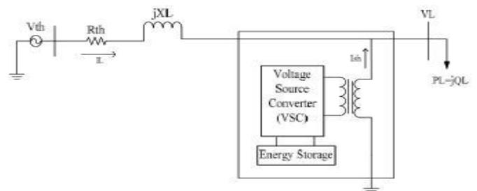
With voltage of 1p.u. at load point, DSTATCOM forces load to operate always at rated power. The STATCOM used in distribution systems is called DSTATCOM (Distribution-STATCOM). It can exchange both active and reactive power with the distribution system by varying the amplitude and phase angle of the converter voltage with respect to the line terminal voltage
