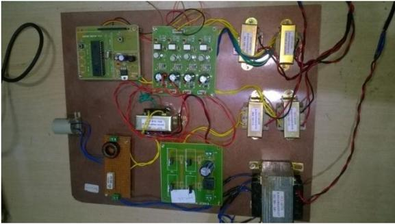
**Figure 3.3.** Hardware model of D-Statcom
