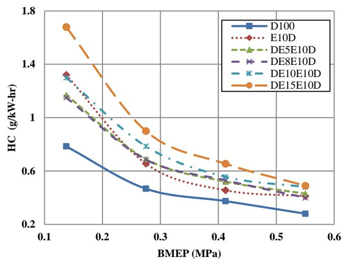
**Figure 6.** Variation of Unburned Hydrocarbon emission with respect to BMEP
