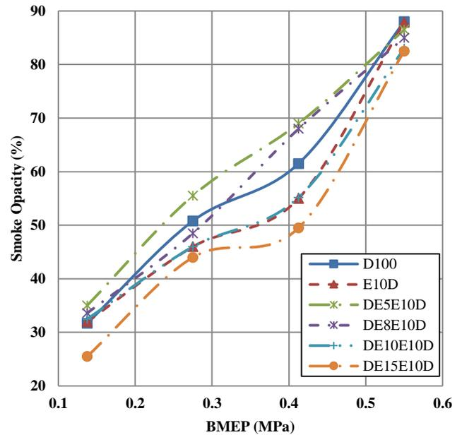
**Figure 3.** Variation of Smoke emission with respect to BMEP
