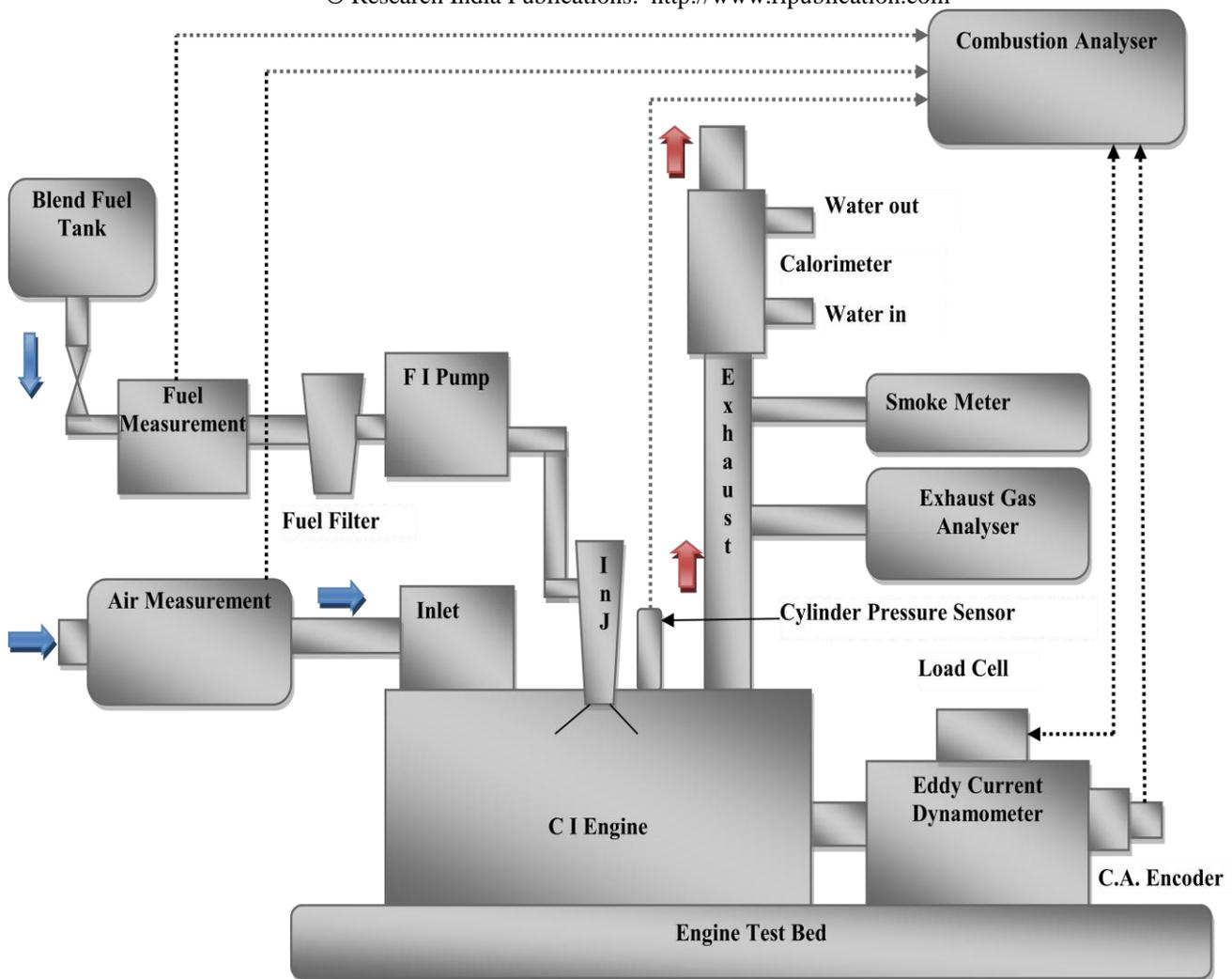
**Figure 1.** Schematic block diagram of engine test rig
