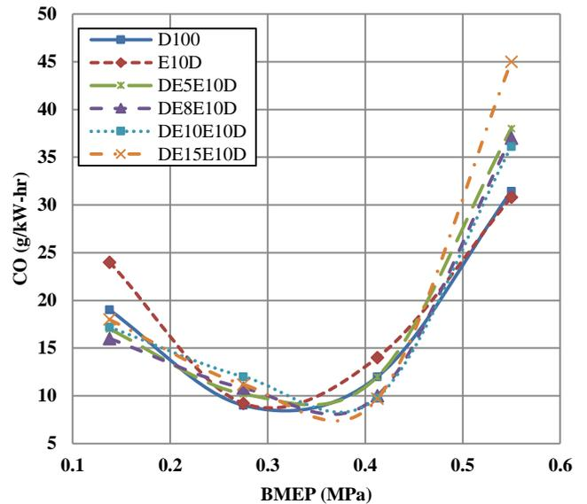
**Figure 5.** Variation of CO emission with respect to BMEP
