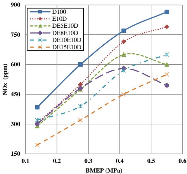
**Figure 4.** Variation of NOx emission with respect to BMEP
