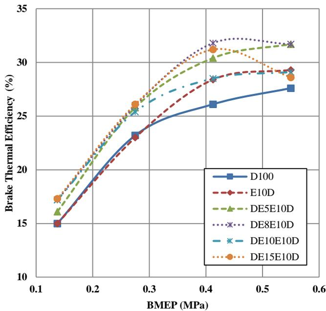
**Figure 2.** Variation of Brake Thermal Efficiency with respect to BMEP.
