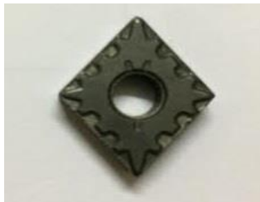
Figure 2. Multi-layer Al-Ti-N coated carbide insert using Thermal Evaporation Technique
