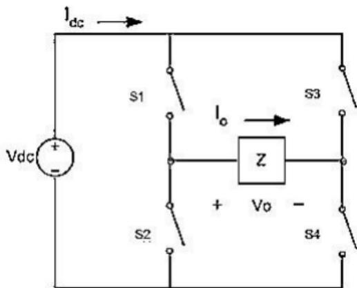
Using the nomenclature above, the switches S1 and S2 should never be closed at the same time, as this would cause a short circuit on the input voltage source. The same applies to the switches S3 and S4. This condition is known as shoot-through. Its basic configuration is shown in figure. This topology is used in conjunction with either the square wave, or pulse width modulation (PWM) switching schemes. The square-wave switching scheme is a method for controlling the
