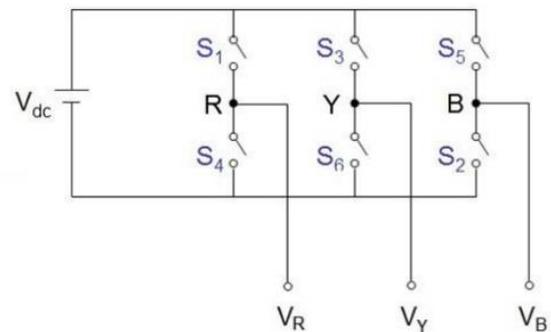
A Basic three phase inverter consists of three legs, each attached to the phase output line. The upper and lower switching transistor are S1 & S4 for R phase, S3 & S6 for Y phase and S5 & S2 for B phase respectively.
