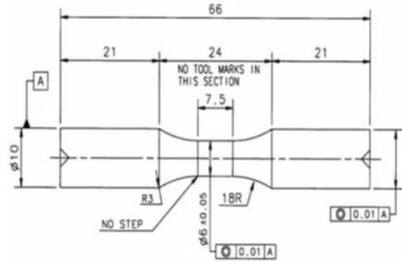
**Figure 1.** The dimensions of the specimen for Rotating bending fatigue specimens test refer to ISO test standard 1143 (1975).
