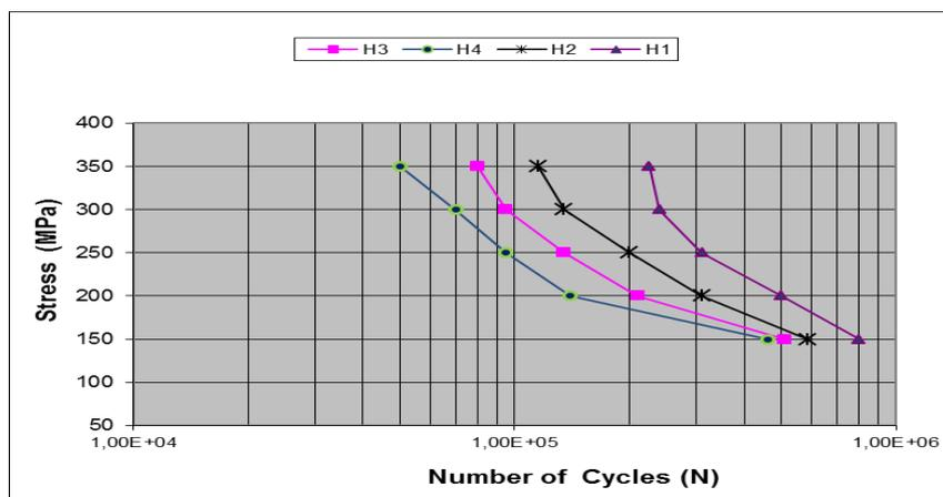
**Figure 3.** Stress versus number of cycles for Specimens after Pack Carburizing
