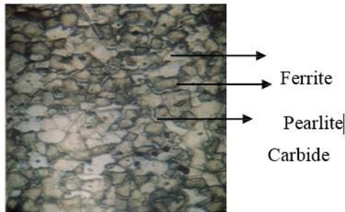
**Figure 5.** Microstructure of specimens uncarburized with 400 times magnification
