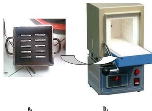
**Figure 2.** Pack Carburizing Process : a.Carburizing Box
