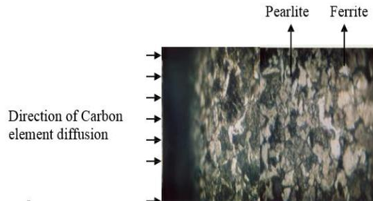
**Figure 7.** Microstructure of specimens Tempering and Quenching in in 30% NaCl solution
