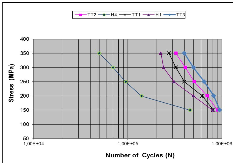
**Figure 4.** Stress versus number of cycles for tempered Specimens after pack carburizing
