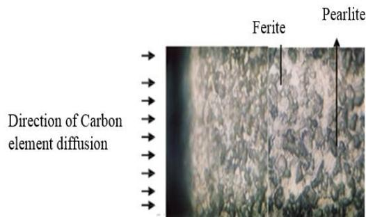
**Figure 6.** Microstructure of specimens after pack carburizing with media carburizer composition 30% PCL shell powder
