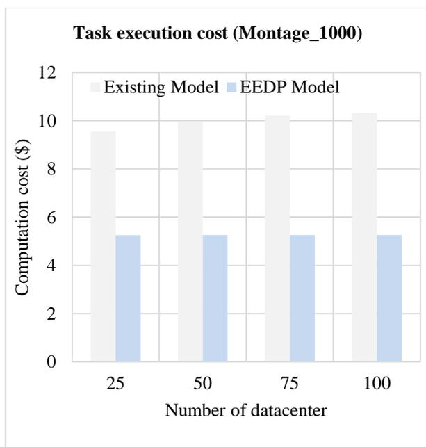
**Figure 4.** Task execution computing cost considering Montage\_1000 dataset
