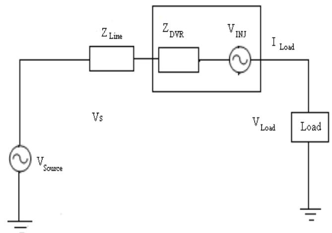
Figure. 2 Equivalent Circuit Diagram of DVR.
