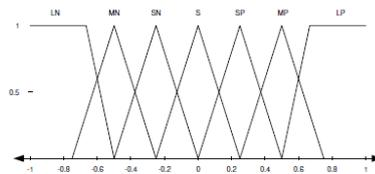
Figure.5 Membership function Input variable “Error”
