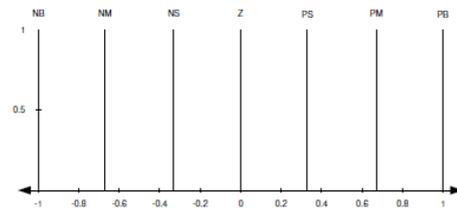
Figure.7 Membership function for output
