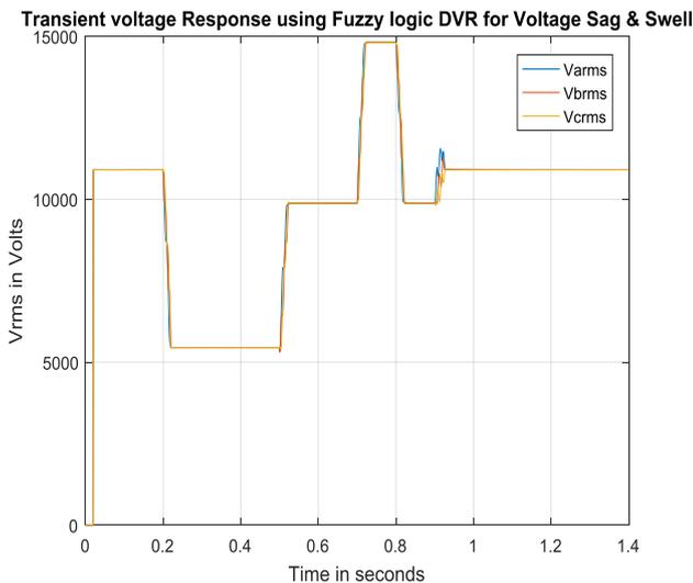
**Figure. 11** Voltage VRMS at the load with Fuzzy logic DVR
