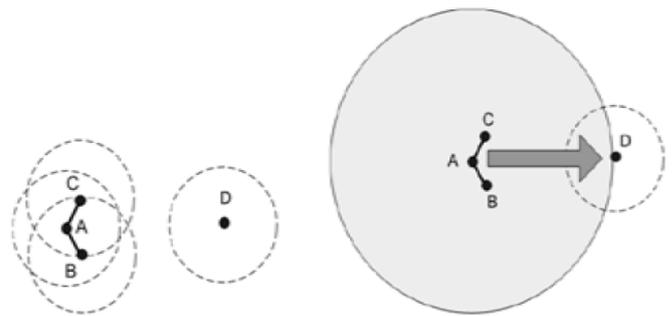
**Figure 1.** Effect of Transmission Range on Network Connectivity
