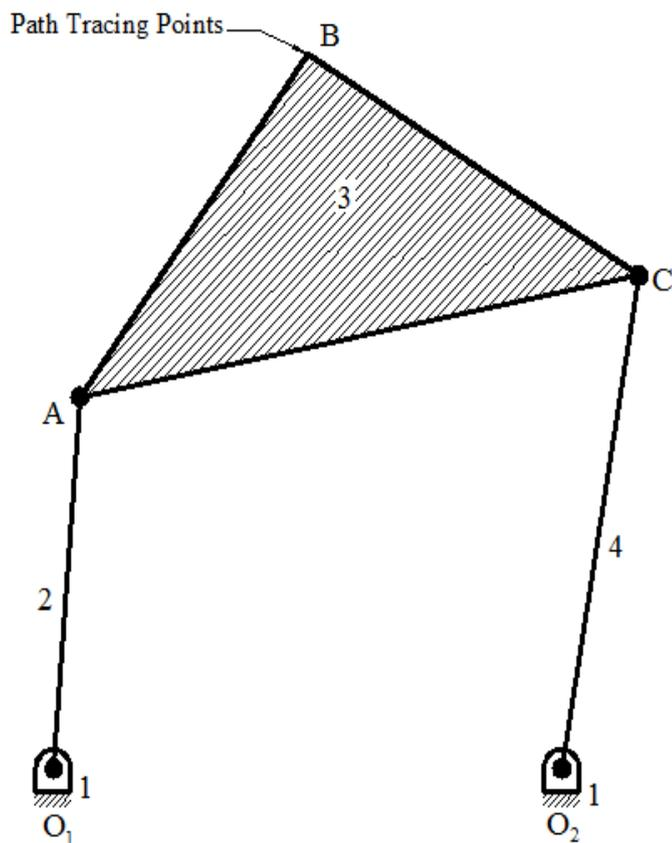
Figure. 1: Configuration of 4-Bar Mechanism
