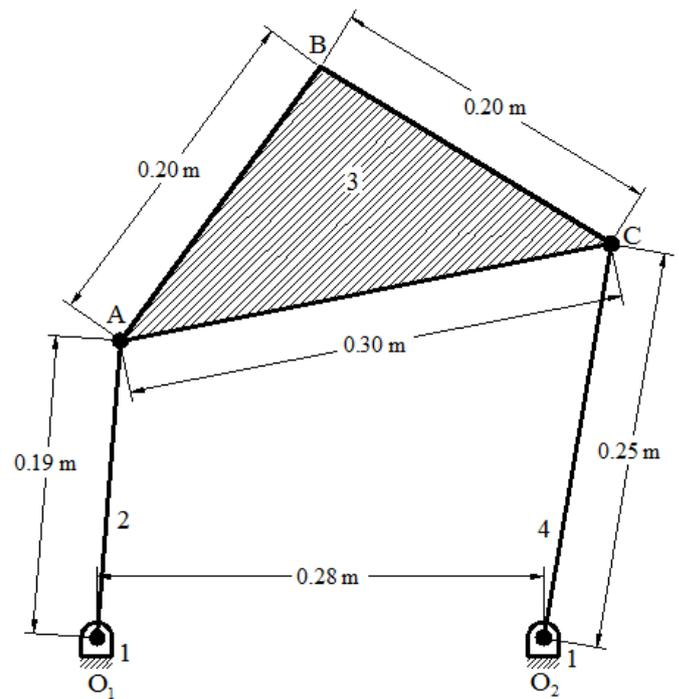
Figure. 2 Dimensional length of 4-Bar Mechanism
