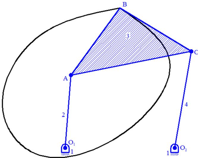
**Figure. 4** Coupler Curve Equation generated by prescribed 4-Bar Mechanism
