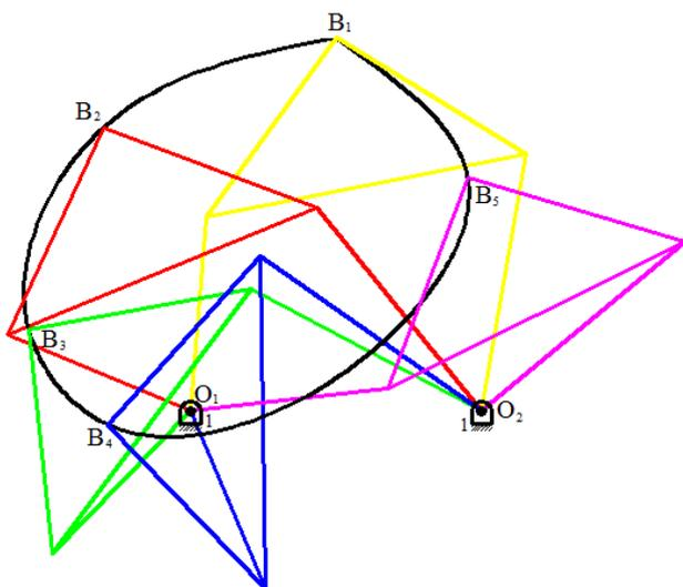
**Figure. 3.** Successive Rotation of Crank link  $O_1A$  of Prescribed 4-Bar Mechanism
