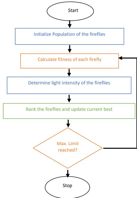
**Figure 4:** Flow diagram for Firefly algorithm
