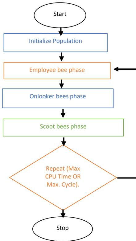
Figure 5: Artificial Bee colony flow diagram
