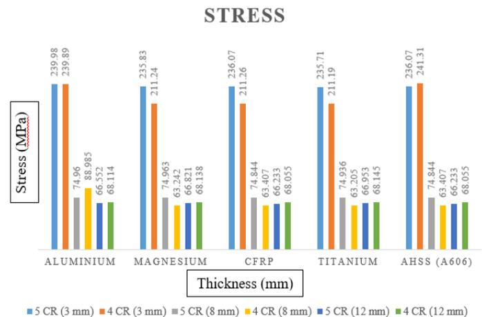
**Figure 11:** Comparison between original and modified chassis stress.
