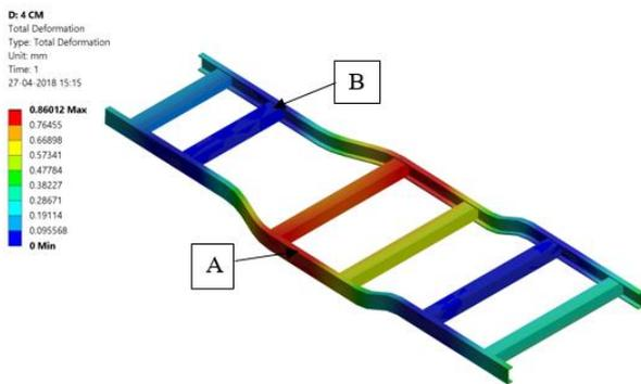
**Figure 12:** Total Deformation-Maximum deflection was observed at point A, which is region at the top of the cross members and minimum was observed at point B.
