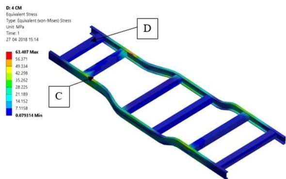
**Figure 13:** Equivalent Stress-Maximum stress was observed at point C, which is on top side of side member and minimum was observed at point D which is on cross members.
