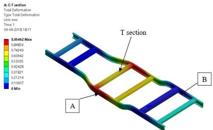
**Figure 15:** Total Deformation-Maximum deflection was observed at point A, which is region at the side of the cross members and minimum was observed at point B below the side members.
