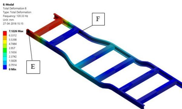
**Figure 14:** Modal Analysis-Maximum deformation was observed at point E, that is on upper side of side member and minimum was observed at point F.
