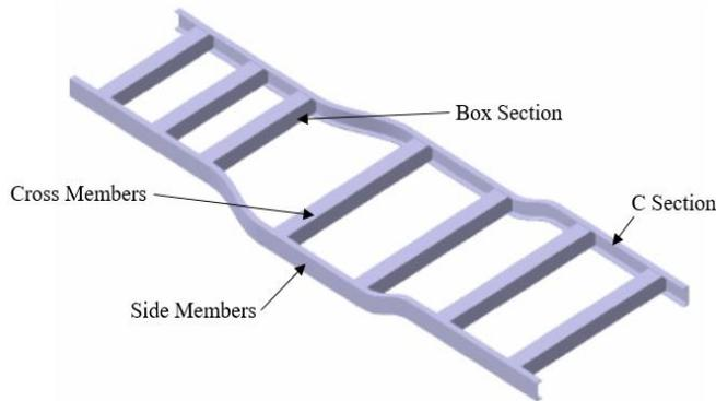
Figure 1: Model of Chassis
