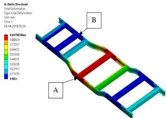
**Figure 7:** Total Deformation-Maximum deflection was observed at point A, that is region joining the cross members and side members and minimum was observed at point B.
