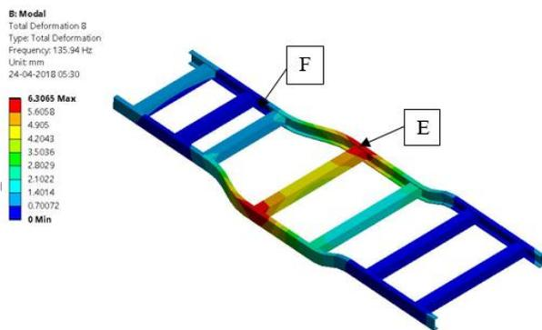
**Figure 9:** Modal Analysis-Maximum deformation was observed at point E, that is on upper side of side member and minimum was observed at point F.
