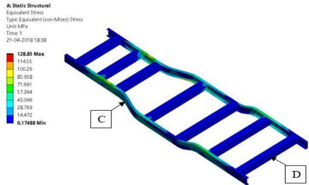
Figure 3: Equivalent Stress-Maximum stress was observed at point C, that is on lower side of side member and minimum was observed at point D that is on cross members.
