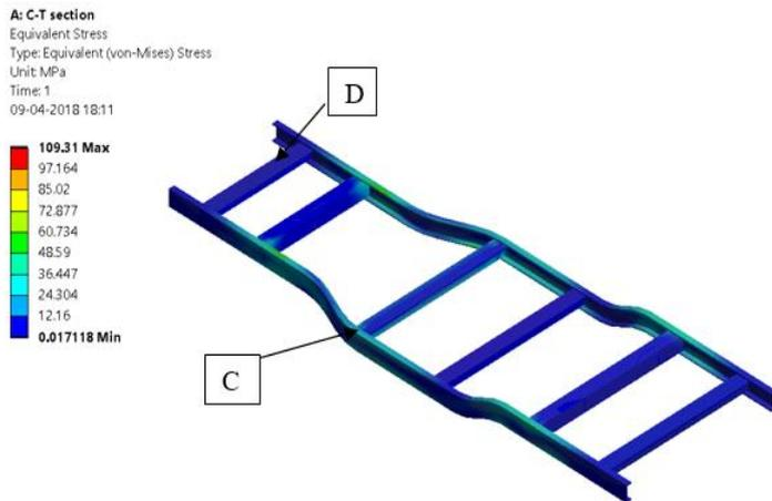
**Figure 16:** Equivalent Stress-Maximum stress was observed at point C, which is on top side of cross members and minimum was observed at point D which is on cross members.
