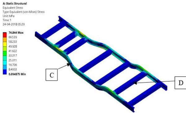
**Figure 8:** Equivalent Stress-Maximum stress was observed at point C, that is on lower side of side member and minimum was observed at point D that is on cross members.
