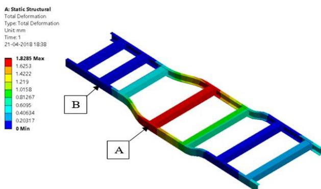
Figure 2: Total Deformation-Point A and B are located at the region joining the cross members and side members.
