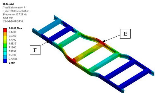
Figure 4: Modal Analysis-Maximum deformation was observed at point E, that is on upper side of side member and minimum was observed at point F.
