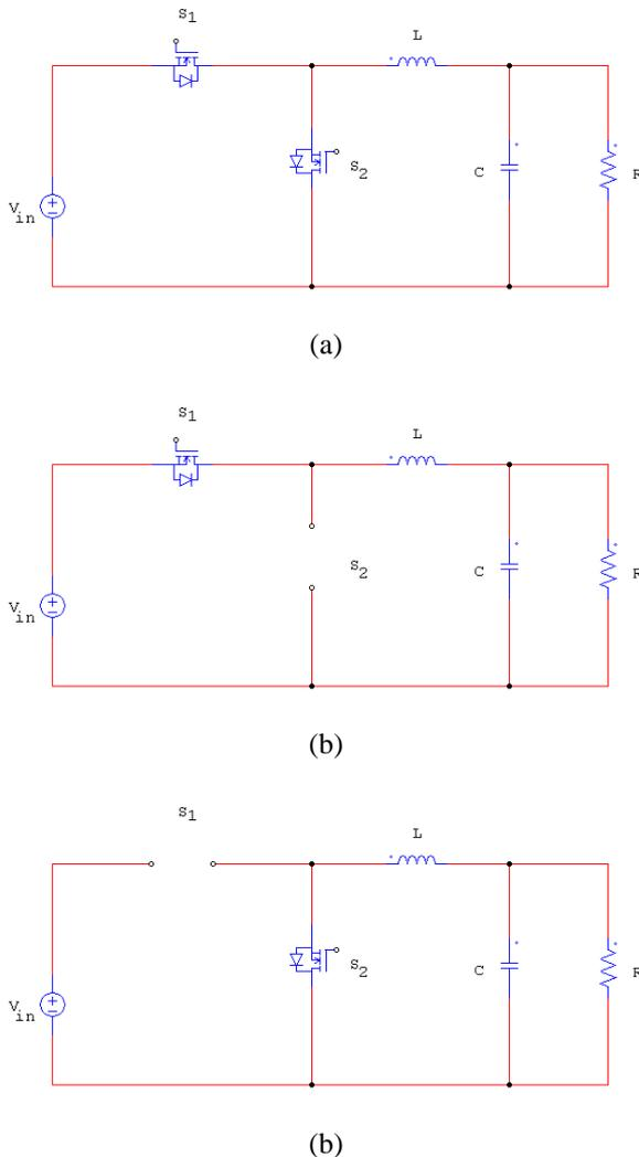
**Figure 1.** SBC power circuit, (a) topology, (b) operation of mode 1 circuit, and (c) operation of mode 2 circuit.
