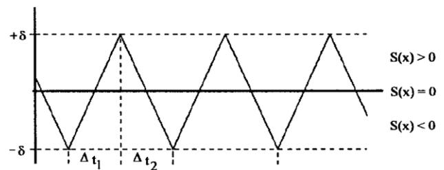
Figure 4. Phase trajectory slides around the surface with allowed HB
