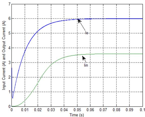
**Figure 11.** SBC Simulated response of average input and output currents with HB based SMC.
