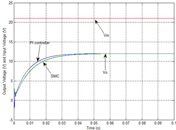
**Figure 10.** SBC Simulated output voltage responses with HB based SMC and PI controller when capacitor variation from 107µF to 150µF.
