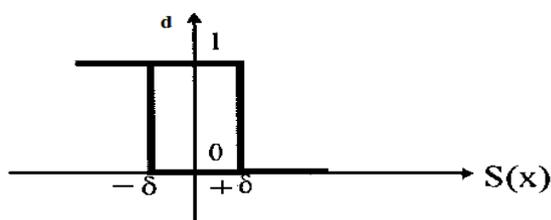
Figure 3. Switching function d.
