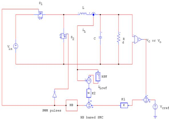
Figure 2. HB based SMC applied to the SBC.
