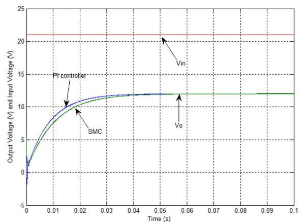
**Figure 9.** SBC Simulated output voltage responses with HB based SMC and PI controller when inductor variation from  $85.5\mu H$  to  $100\mu H$ .
