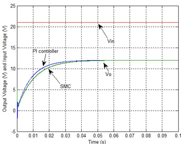
**Figure 5.** SBC Simulated output voltage reponses using HB based SMC and PI controller in start-up transient region for  $V_{in} = 21V$ .
