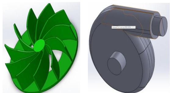
**Figure 3.** Assembly of blower
