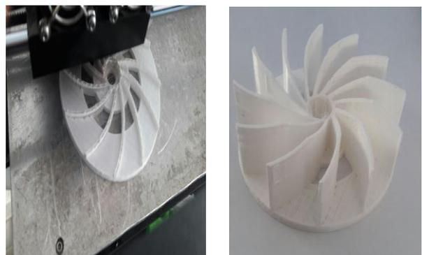
Figure 12. 3D printing process of impeller
