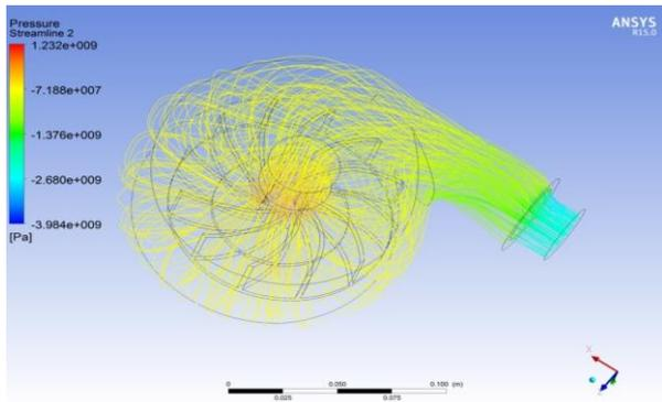
Figure 5. Pressure streamline
