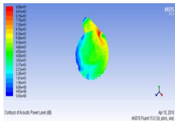
Figure 8. Power level contour
