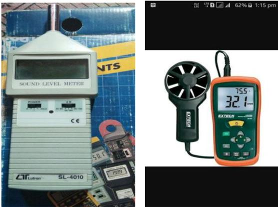
**Figure 13.** Decibel meter and Anemometer
