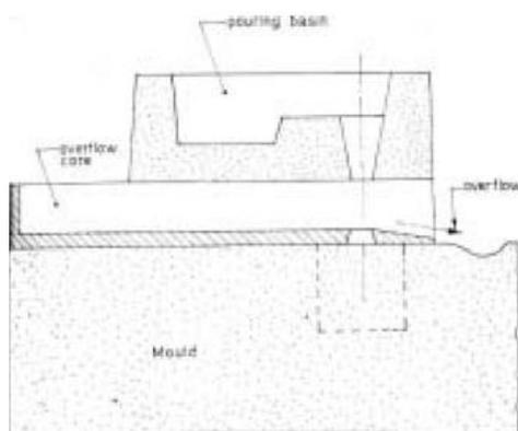
**Figure 2.** Diagram for the volume deficit experiment for cube shape casting
