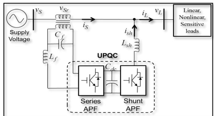
Figure 1. Conventional UPQC consist of shunt and series converters
