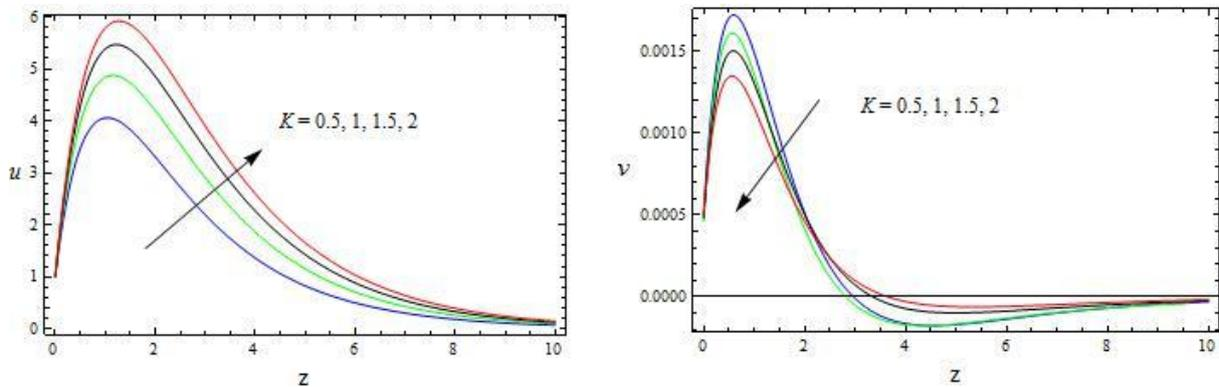
**Figures 4.** The velocity Profiles for  $u$  and  $v$  with  $K$
