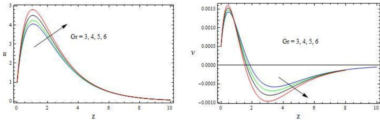
**Figures 5.** The velocity Profiles for  $u$  and  $v$  with  $Gr$
