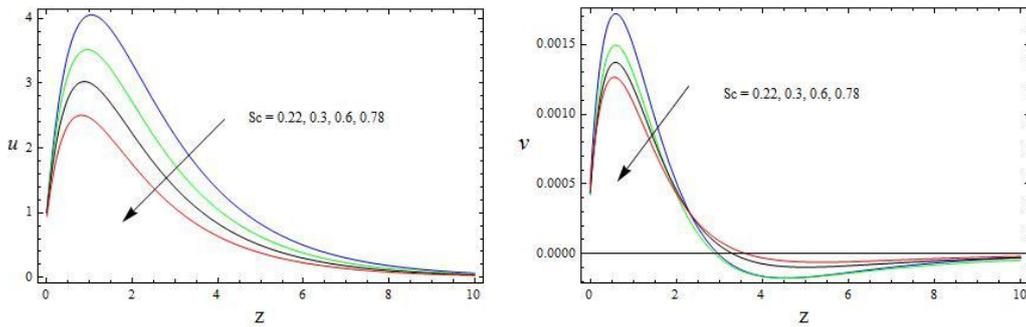
**Figures 10.** The velocity Profiles for  $u$  and  $v$  with  $Sc$
