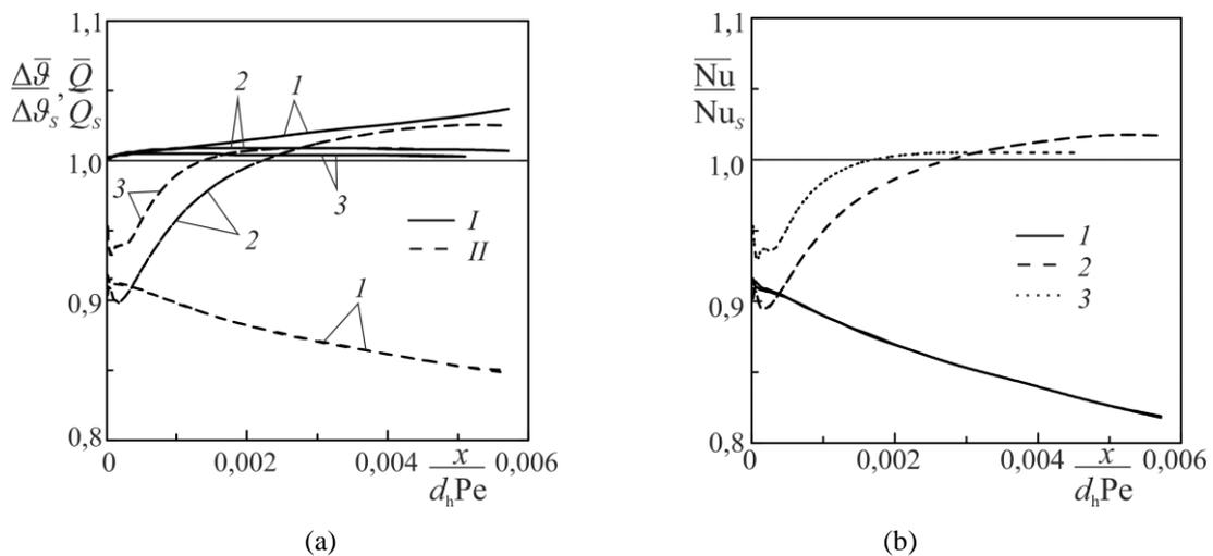
**Figure 5:** change of average temperatures in time of a difference, a thermal stream (a) and Nusselt number (b) to their stationary values when  $A = 1$  and  $Pr = 35$ .  $1 - S \rightarrow 0$ ;  $2 - S = 4$ ,  $3 - 16$ .
