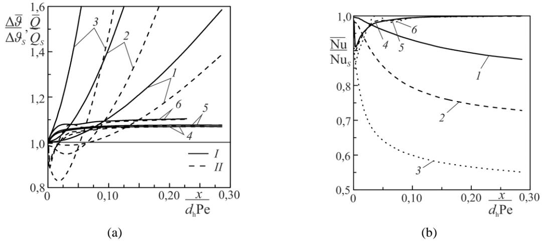
**Figure 4:** change of temperature average in time difference, a thermal stream (a) and Nusselt number (b) to their stationary values when  $Re = 1000$  и  $Pr = 0,7$ .  $1, 2, 3 - S \rightarrow 0$ ;  $4, 5, 6 - S = 16$ ;  $1, 4 - A = 0,25$ ;  $2, 5 - A = 0,5$ ;  $3, 6 - A = 1,0$ ;  $I - \Delta\bar{\vartheta} / \Delta\vartheta_s$ ,  $II - \bar{Q} / Q_s$ .
