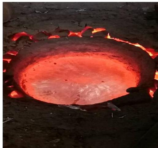
**Figure 2:** Al7075 alloy Melt at desired Temperature
