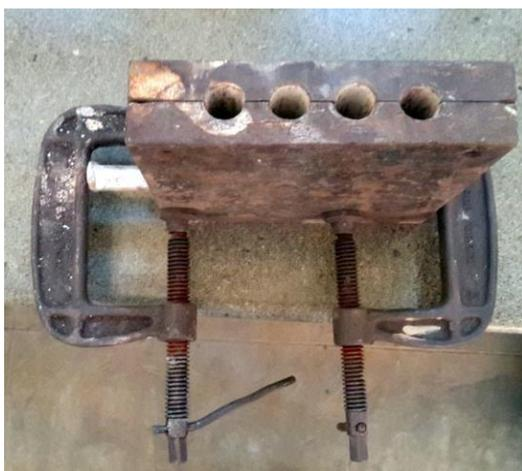
**Figure 1:** The Die set after Pre Heating
