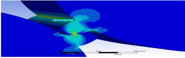
Figure 9: 3-D Von Mises stresses on the root of tooth.
