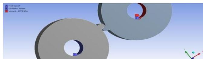
Figure 8: Applied Boundary Condition
