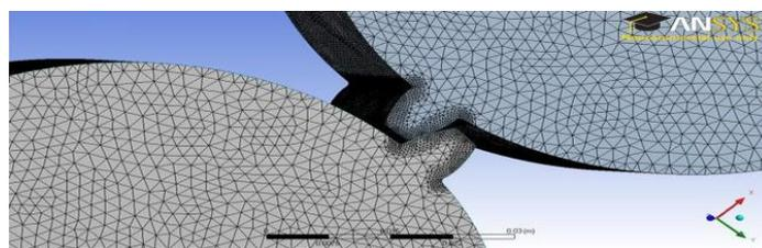
Figure 7: A three dimensional FEM model with mesh
