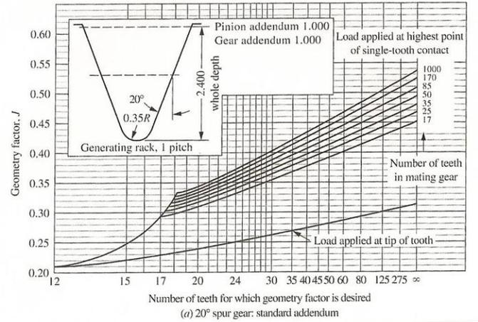
Figure 13: Spur-gear geometry factors, Source: The graph is from AGMA. The graph is convenient for design purposes.
