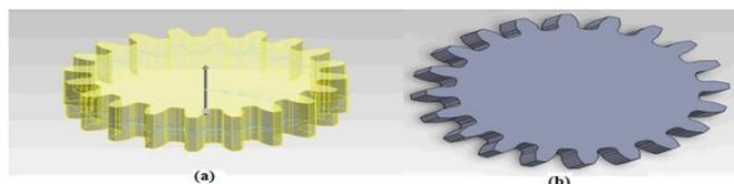
Figure 4: (a) and (b): Involute spur gear solid model.
