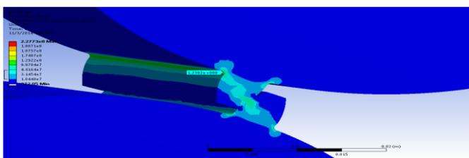
**Figure 14:** 3-D Von Mises (bending) stress at the root of the tooth.
