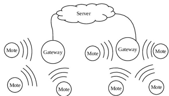
Figure.1. Topology of LoRaWAN
