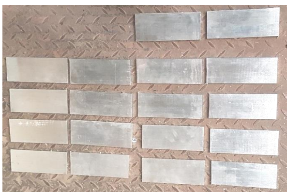
Figure 2. Sheared pieces of AA 7075 Sheet material
