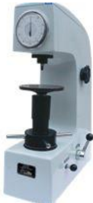
Figure 6. Rockwell hardness tester
