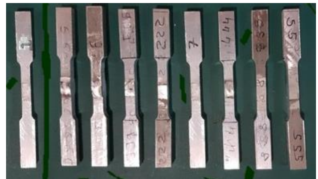
Figure 8. Prepared tensile specimen as per ASTM E8 Standard
