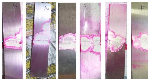
Figure 4. Dye penetrant test samples 1
