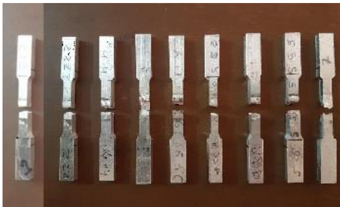
Figure 9. Tensile specimens after tensile testing
