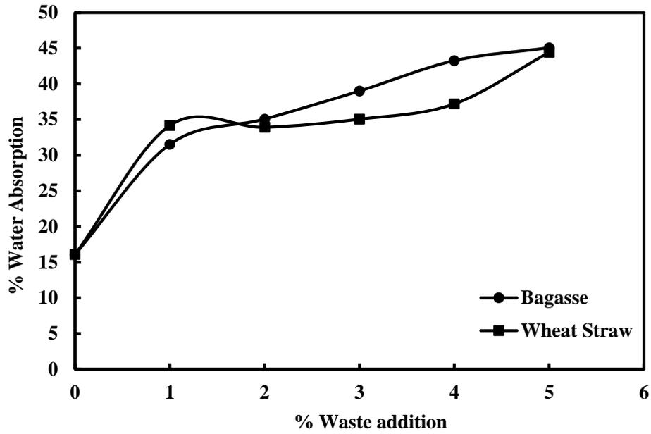
Figure 4: Effect of Percent bagasse and wheat straw on Water Absorption
