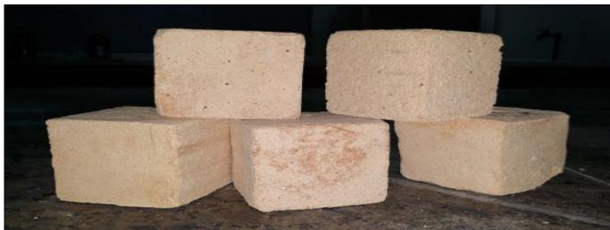
Figure 2: Clay bricks samples after firing
