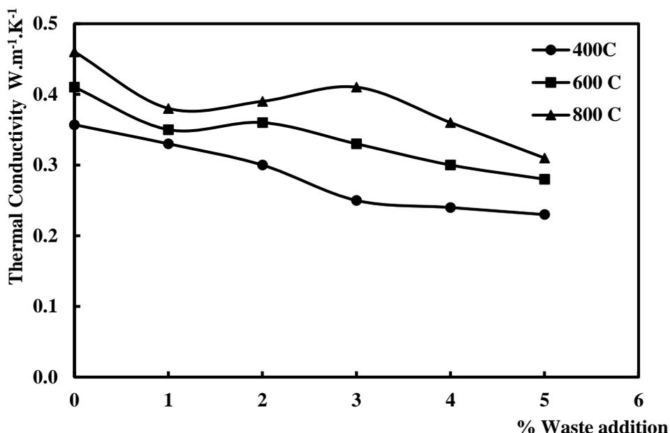
Figure 8: Effect of Percent wheat straw on Thermal conductivity
