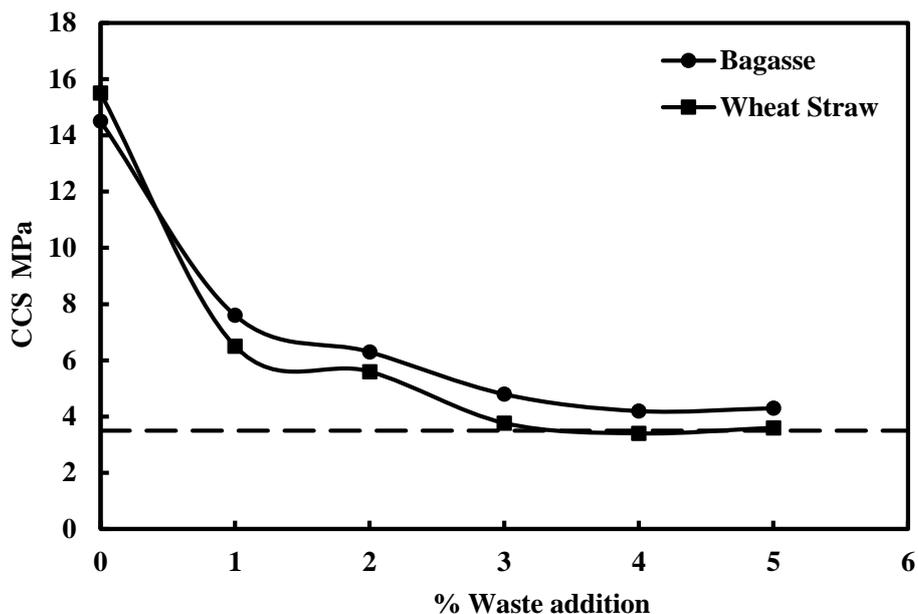
Figure 6: Effect of Percent bagasse and wheat straw on Cold Crushing Strength
