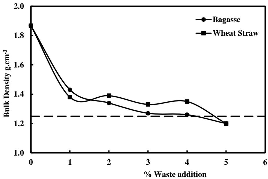
Figure 5: Effect of Percent bagasse and wheat straw on Bulk density
