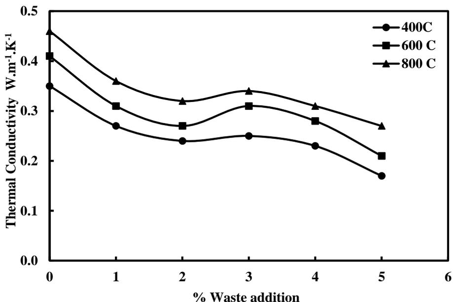
Figure 7: Effect of Percent bagasse on Thermal conductivity
