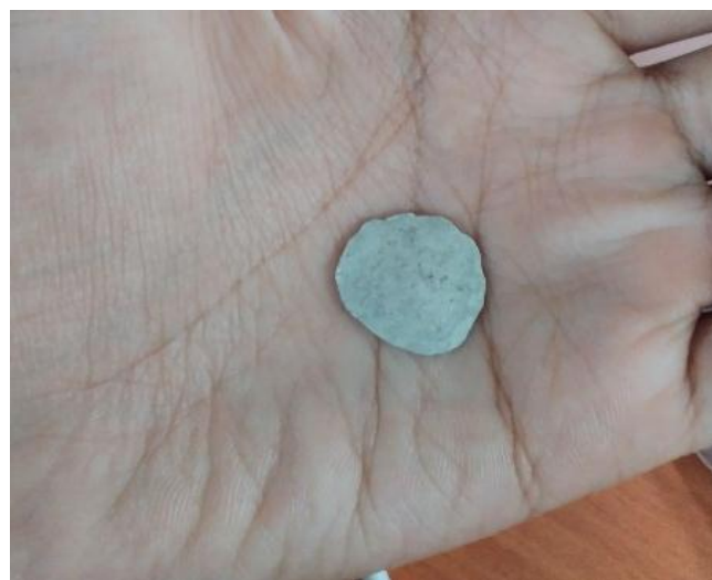
Figure 2. Bullion result in gold extraction from tailings waste by heap leaching method and silver nitrate material assistance.
