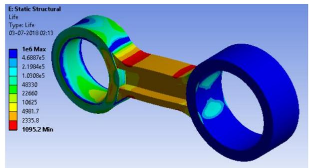
Figure 3. Uncoated Fatigue Life
