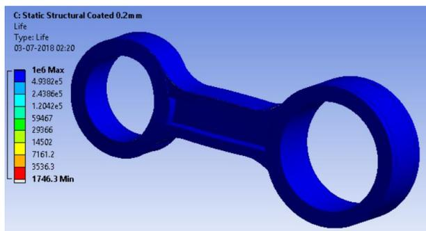
**Figure 4.** Fatigue Life YSZ Plasma Coated Component.
