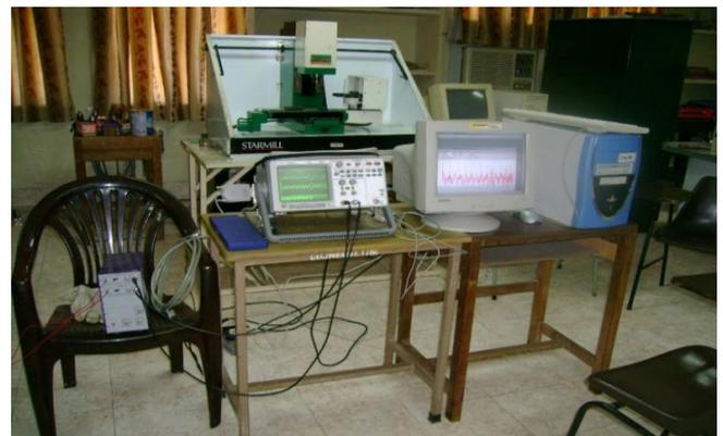
Figure 2. Experimental Setup for Measuring Tool Vibration
