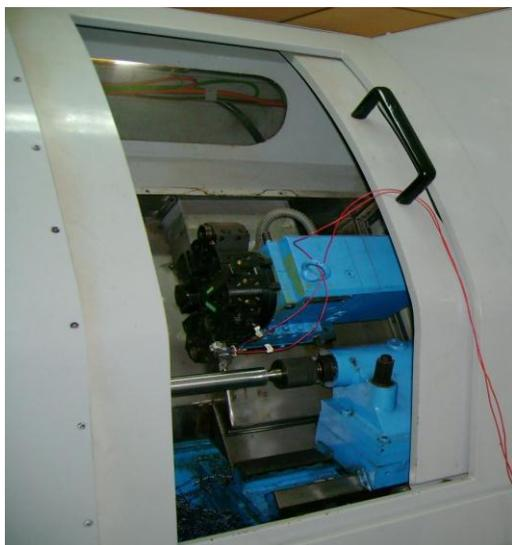
Figure 1. View of Tool Holder, Insert & Sensor
