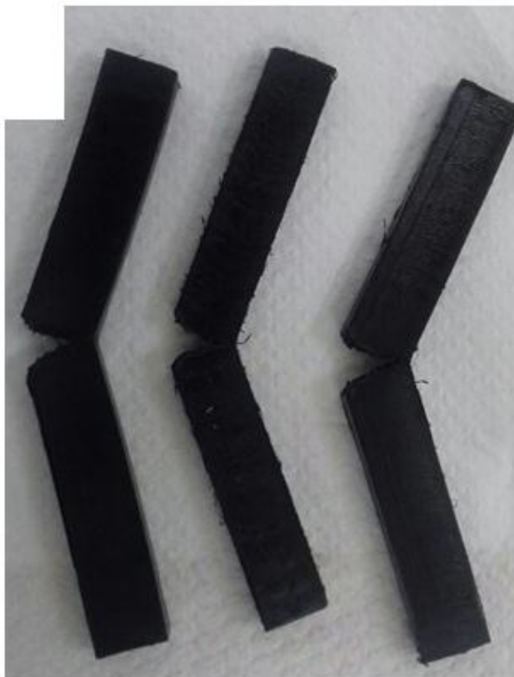
Figure 8. HDPE samples with notch after impact testing at RT carried out in Mechanical Engineering Laboratory, NEU) (10mm (width)× 4mm (thickness)× 80mm(length)) with 2mm depth (V)
