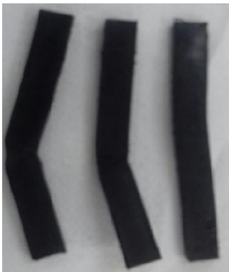
Figure 7. HDPE samples without notch after impact testing at RT carried out in Mechanical Engineering Laboratory, NEU (10mm (width)× 4mm (thickness)× 80mm(length))
