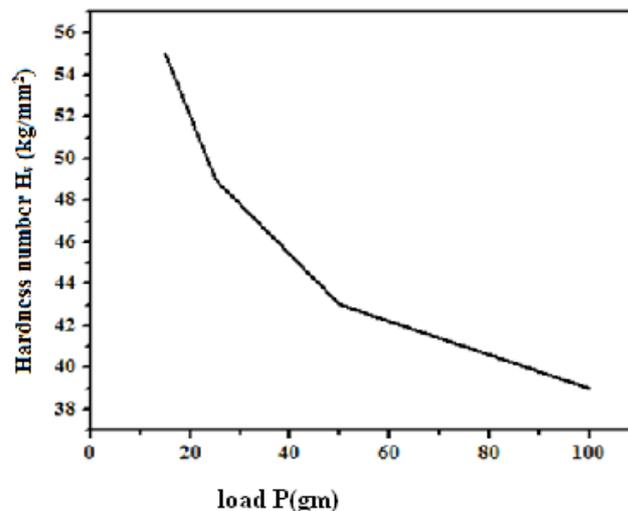
Figure 6. shows the relation between Vickers hardness number vs load of LTCC.
