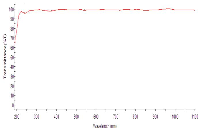
Figure 4. Transmission spectrum of LTCC single crystal
