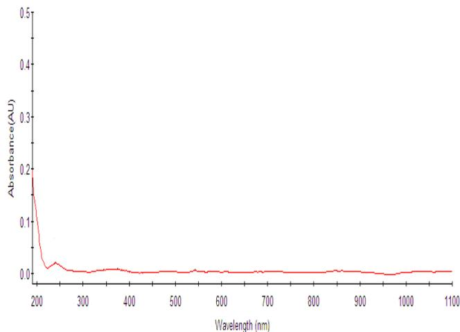
Figure 5. Absorption spectrum of LTCC crystal
