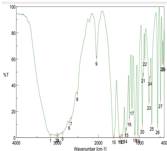
Figure 3. FT – IR spectrum of LTCC crystal.
