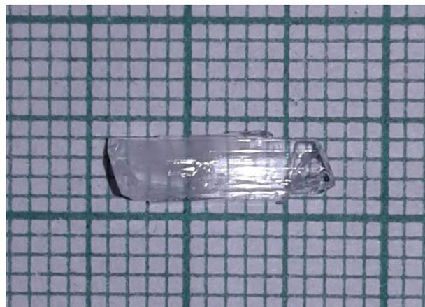
**Figure 1.** Photograph of as grown single crystal of LTCC
