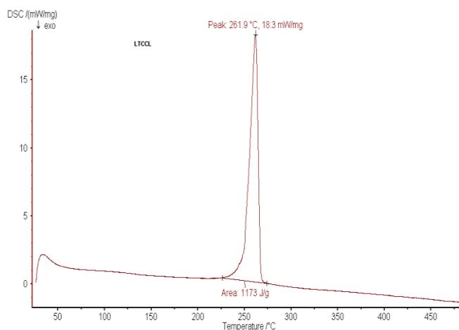
Figure 7. DSC of LTCC single crystal
