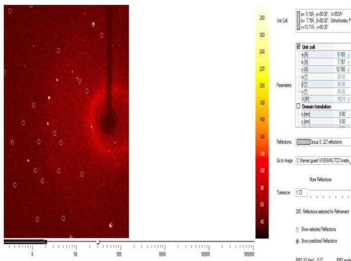
Figure 2. Single crystal XRD pattern
