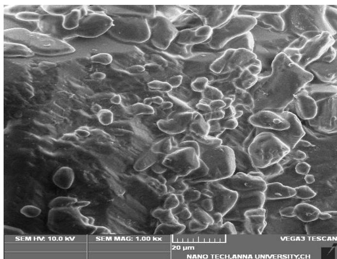
**Figure 10.** FE-SEM of LTCC crystal
