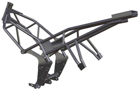
Figure 1. 3D CAD geometry model of X71A framebody
