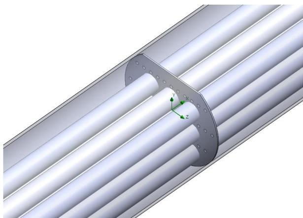
**Figure 11:** Baffle gap 15mm along with spherical dimples on baffles
