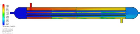
**Figure 13:** Interior fluid temperature (front plane cut section)
