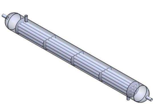
Figure 7: View of tubes and baffles
