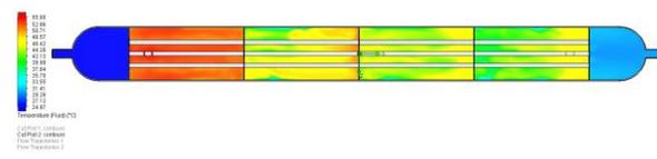
**Figure 14:** Interior fluid temperature (top plane cut section)
