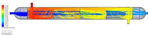
**Figure 15:** Interior fluid flow pattern (flow trajectories)
