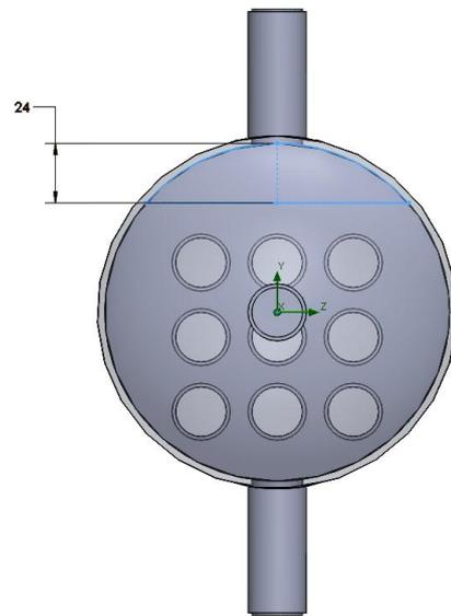
Figure 9: Baffle gap reduced from 34 mm to 24mm
