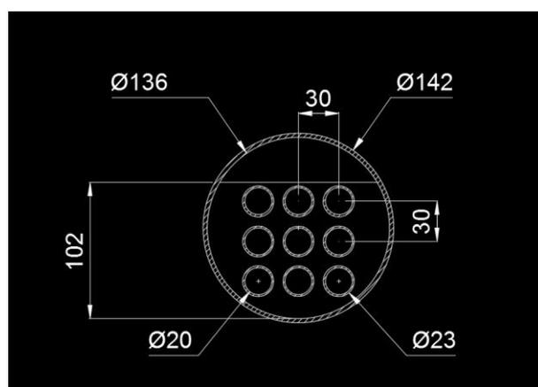
**Figure 5:** 8 Dimensions of shell, tube and baffle
