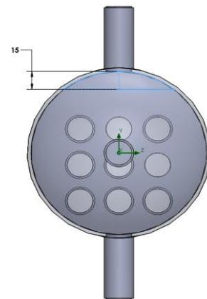
Figure 10: Baffle gap reduced from 34 mm to 15mm
