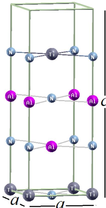
**Figure 1.** Unit cell for TiN/AlN/TiN interlayer obtained after relaxation process.
