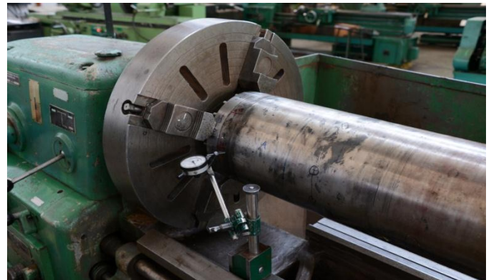
Figure 4. Truing of Rocket Motor on Lathe
