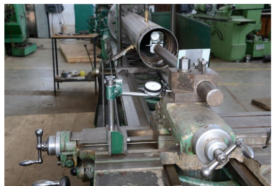
Figure 5. Attachment of boring bar, dial gauge, plane mirror
