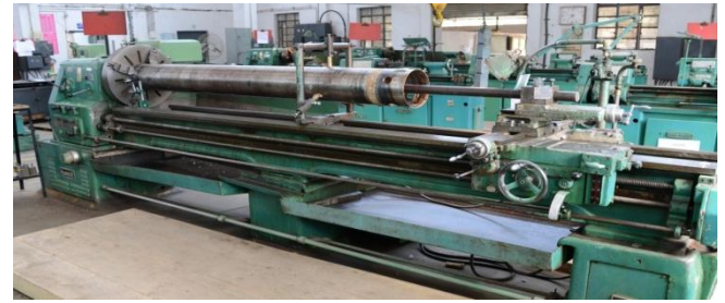
Figure 3. Rocket Motor mounted on Lathe
