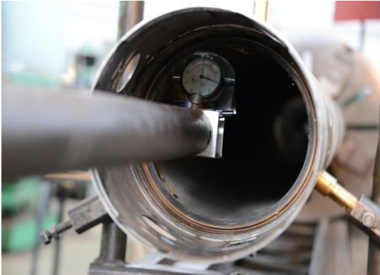
Figure 6 A. Measurement reading being taken at a given location
