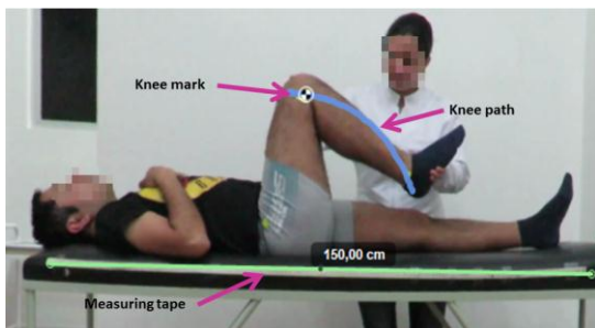
Figure 2. Path developed by the knee.
