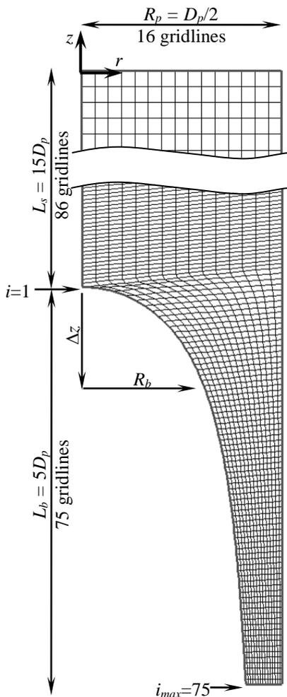
**Figure 2:** Schematic Diagrams of an Employed Grid in a Domain Forces Given by the Simulator
