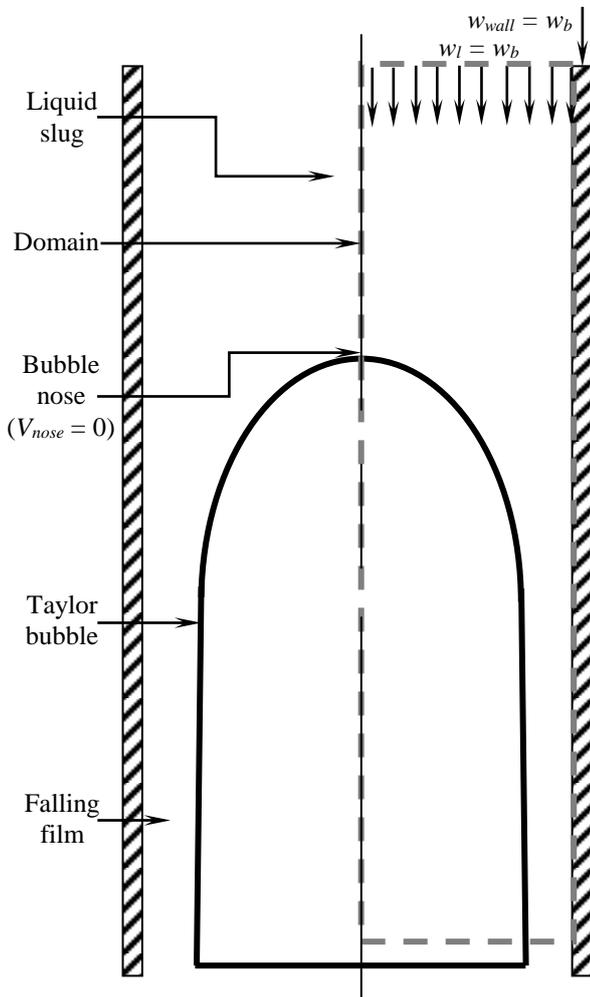
**Figure 1:** Schematic Diagram of a Slug Flow in a Stagnant Liquid with respect to the Taylor Bubble Nose
