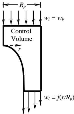
**Figure 4:** Diagram of Mass Influx and Efflux on the control surfaces of a Taylor Bubble Unit
