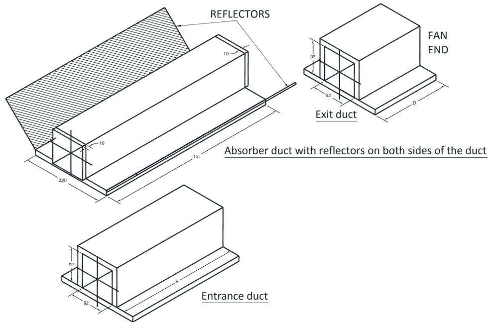
**Figure 3.** Isometric view of the air heater configuration with side reflectors
