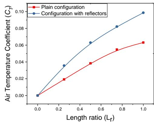
**Figure 8.** Temperature coefficient of absorber air along the flow path for lower mass flow rate  $m_1$
