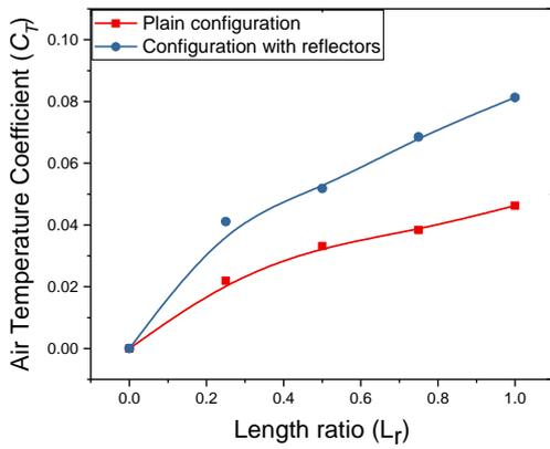
**Figure 9.** Temperature coefficient of absorber air along the flow path for intermediate mass flow rate  $m_2$
