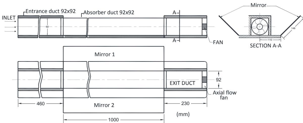
**Figure 2.** Schematic diagram of the air heater configuration with side reflectors
