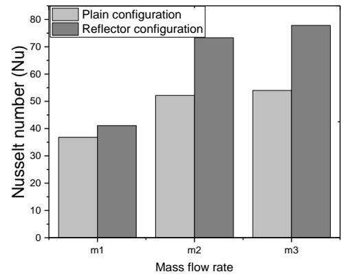
**Figure 7.** Nusselt number for the two configurations corresponding to the three mass flow rates
