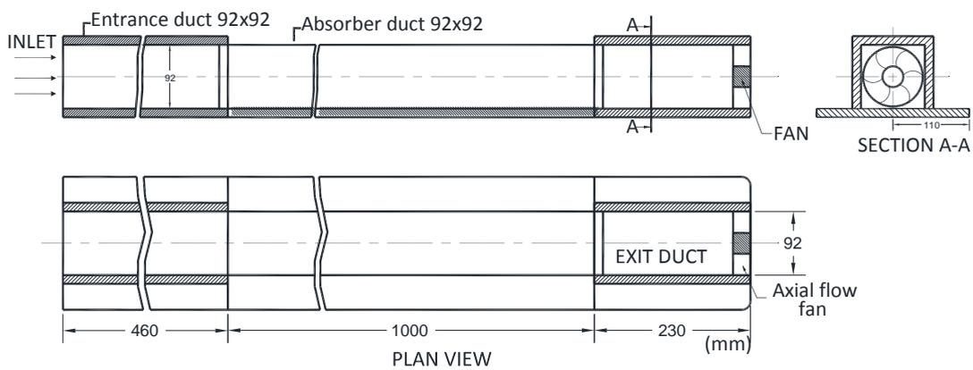
**Figure 1.** Sketch of the of the configuration without reflectors
