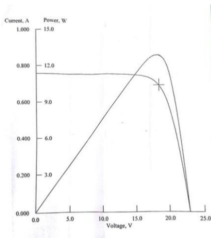
**Figure 4.** The voltage and current characteristics of the 10W solar panel.
