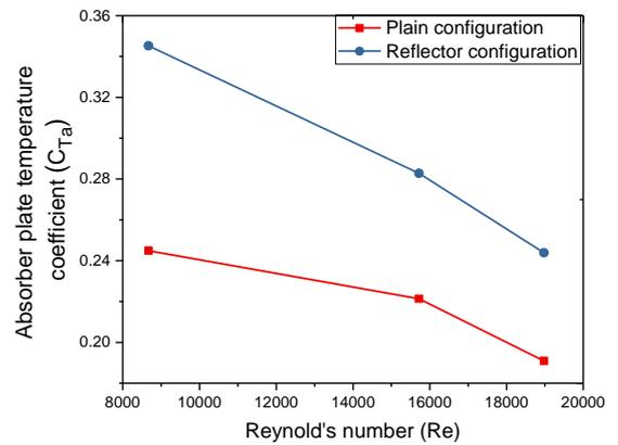
**Figure 11.** Plot of absorber plate's temperature coefficient with respect to Reynold's number.
