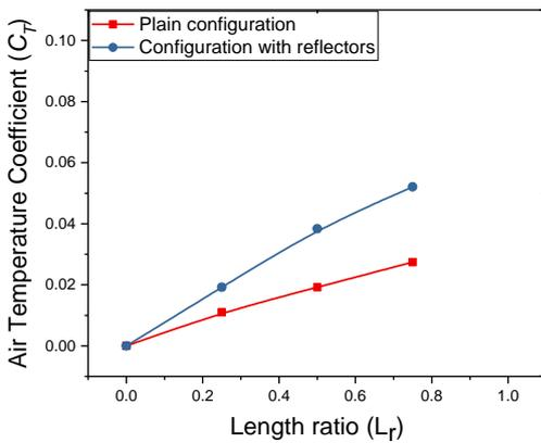
**Figure 10.** Temperature coefficient of absorber air along the flow path for higher mass flow rate  $m_3$
