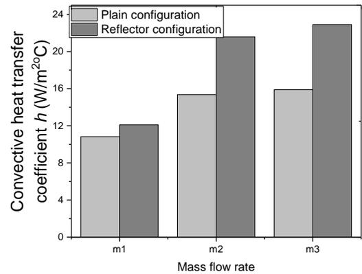
**Figure 6.** Convective heat transfer coefficient for the two configuration corresponding to the three mass flow rates.
