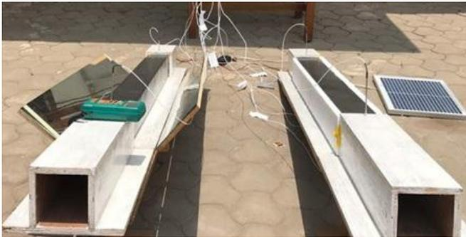
**Figure 5.** Image showing the two air heaters exposed to solar radiation
