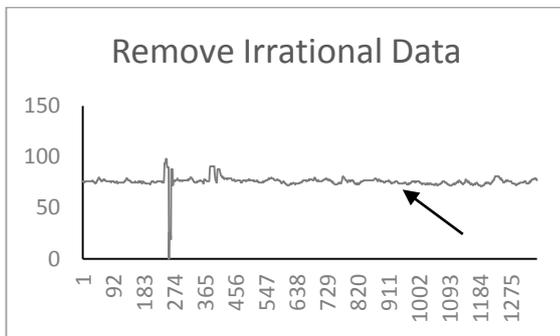
**Figure 2.** Remove irrational data is to eliminate impossible data. In the picture the variance is too small (variation less than 5BPM), so it is not possible.
