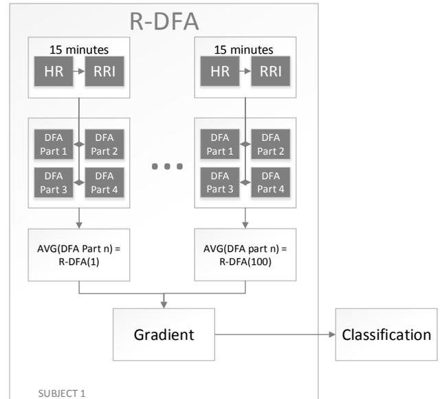
**Figure 10:** The block diagram of R-DFA uses a gradient from R-DFA 1 to n. Gradients can show trends or tendencies of the subject.
