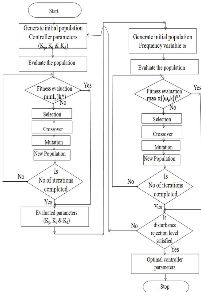
**Figure 4:** Flow chart of design of  $H_\infty$  controller by GA.
