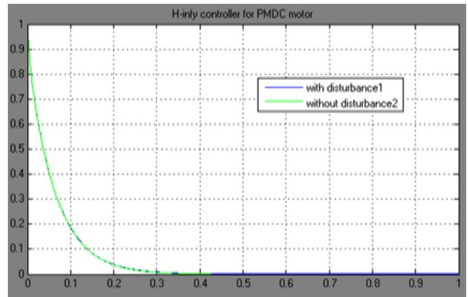
**Figure 10:** Error response (speed) of PMDC motor with controller
