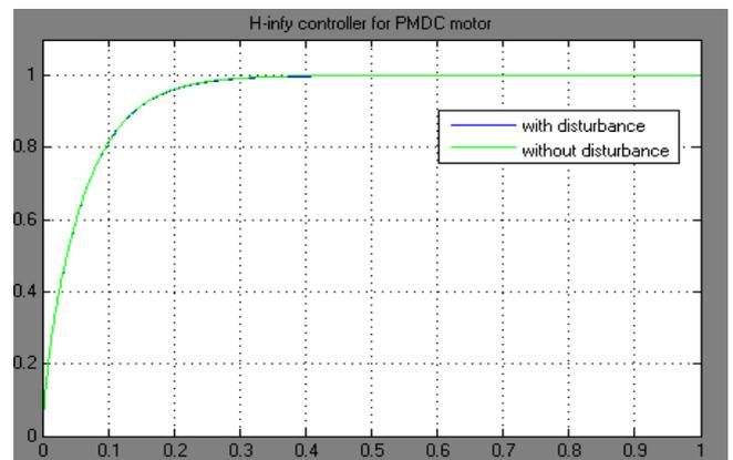
**Figure 11:** Step response (speed) of PMDC motor with and without controller
