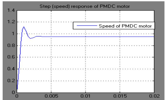
Figure 5: Step (speed) response of PMDC motor
