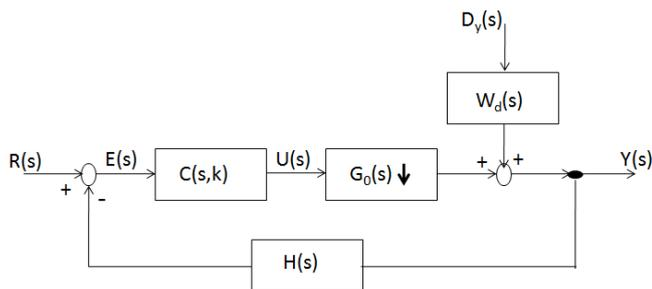
Figure 2: Control system with disturbance.
