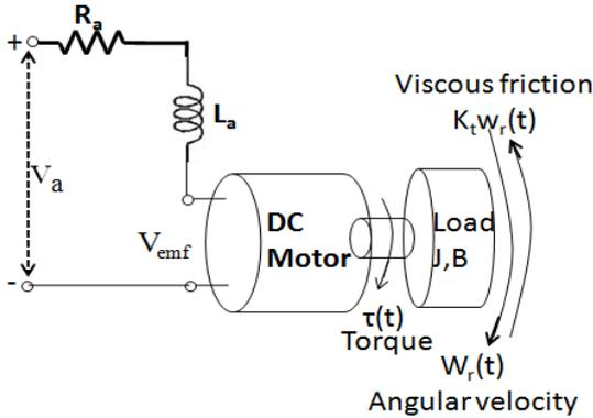
**Figure 1:** Equivalent circuit diagram of PMDC motor.
