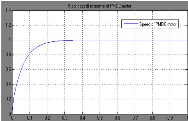
**Figure 7:** Step (speed) response of PMDC motor with controller
