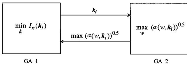
Figure 3: Representation of  $H_{\infty}$  controller by GA
