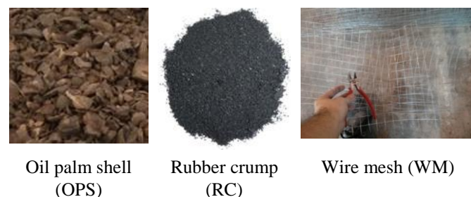
Figure 1. Oil palm shell, rubber crump, and wire mesh for slab reinforcement
