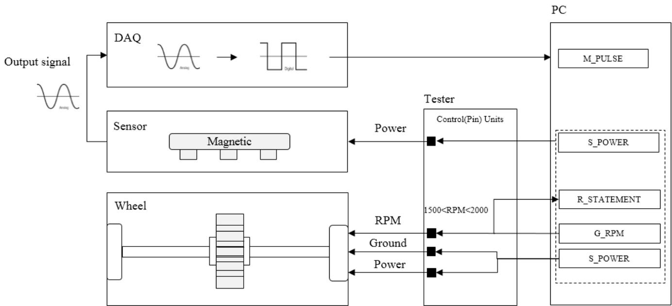
**Figure 5.** The configuration of the speed sensor test
