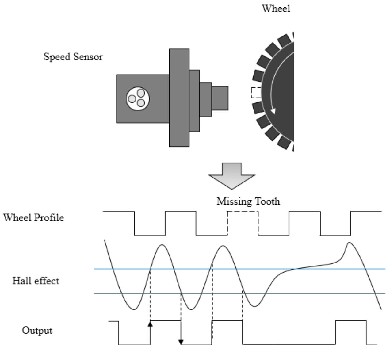
Figure 2. Measuring method of a wheel speed sensor
