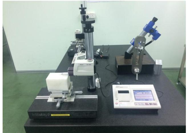
**Figure 14:** Portable Surface Roughness Tester, SJ-401
