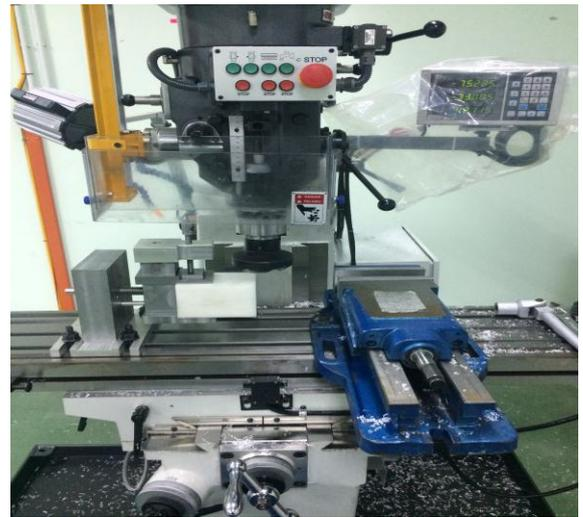
**Figure 8:** Work piece clamp using flexible clamping
