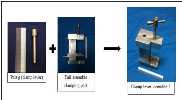
**Figure 6:** Clamp lever assemble 2
