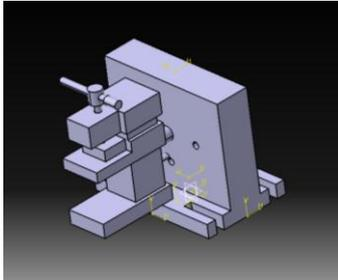
**Figure 1:** Design of flexible clamping using CATIA software
