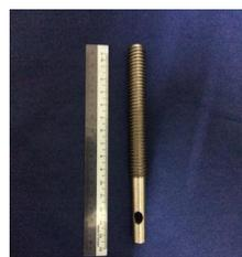
Figure 18: Developed of part c (rod)
