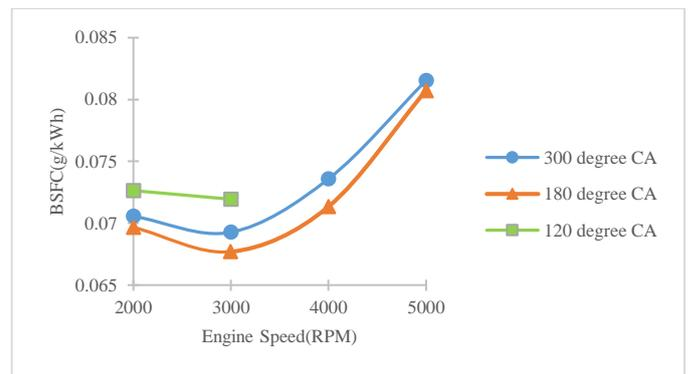
**Figure 3:** BSFC against engine speed at various injection timings
