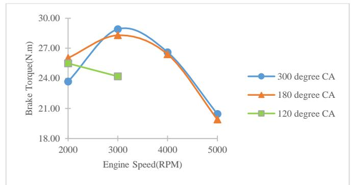
**Figure 2:** Brake-torque against engine speed at various injection timings
