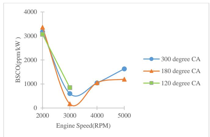
**Figure 5:** BSCO against engine speed at various injection timings
