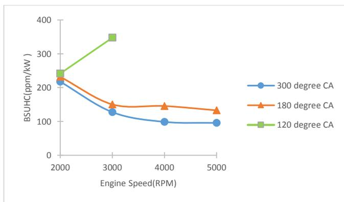
**Figure 6:** BSUHC against engine speed at various injection timings.
