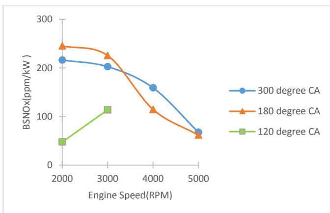
**Figure 4:** BSNOx against engine speed at various injection timings.
